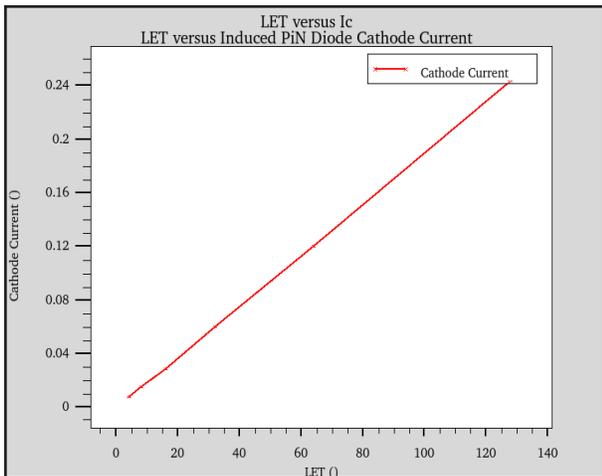
Figure 6. Conversion between Induced Cathode Current in Figure 5 and LET Value.
