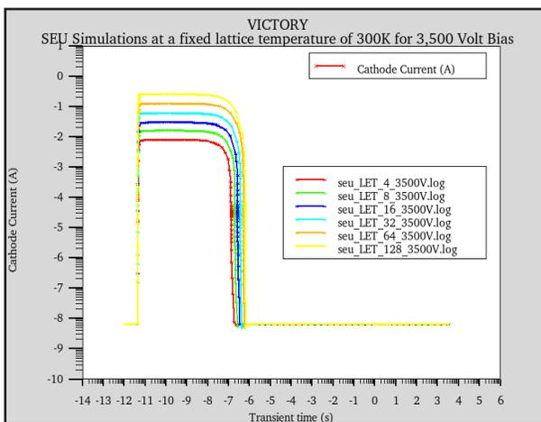
Figure 9. The same simulations as Figure 8, but without localized lattice heating and a substrate temperature of 300K.
