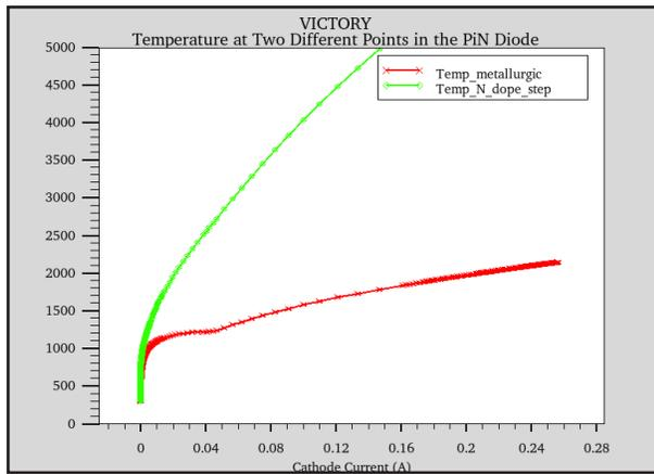
Figure 3. Temperatures inside the PiN diode at the metallurgic junction and at the N+ to intrinsic boundary.
