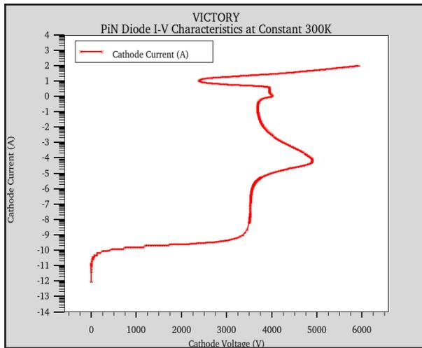
Figure 1. Constant temperature (300K) I-V curves of the 3,500 volt power PiN power diode.
