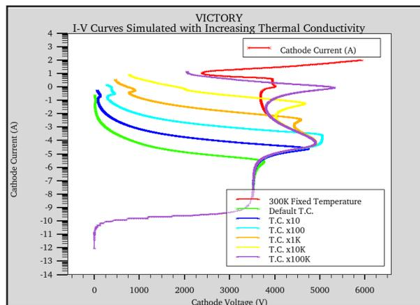
Figure 4. I-V curves using increasing thermal conductivity to emulate non thermal equilibrium effects from an SEU strike.
