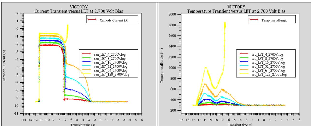
Figure 7. Temperature and Current Simulations of SEU strikes with LET values from 4 to 128 MeV.cm2/mg at a reverse bias of 2,700 volts.
