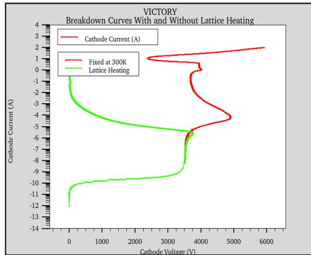
Figure 2. Comparing the no self heating, with a thermal equilibrium curve.
