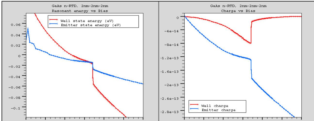
Figure 3. (Left panel) Dependence of the eigen energies in the emitter (blue) and the well (red) on applied bias. (Right panel) Total charge in the emitter (blue) and the well (red).
