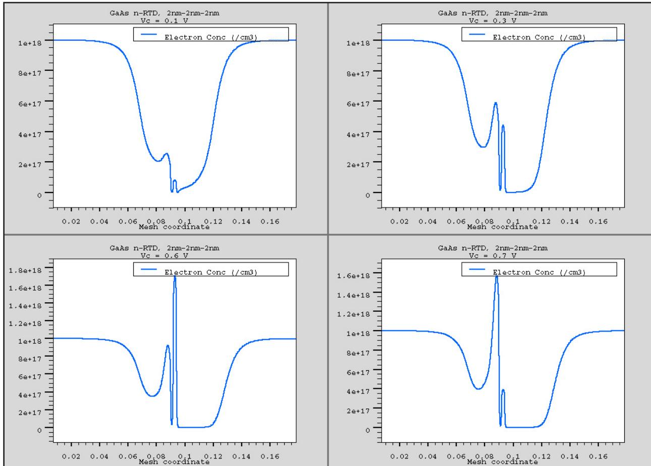
Figure 5. Electron density profiles at biases of 0.1, 0.3, 0.6 and 0.7 V. Note the non-monotonic behavior of the charge in the well.
