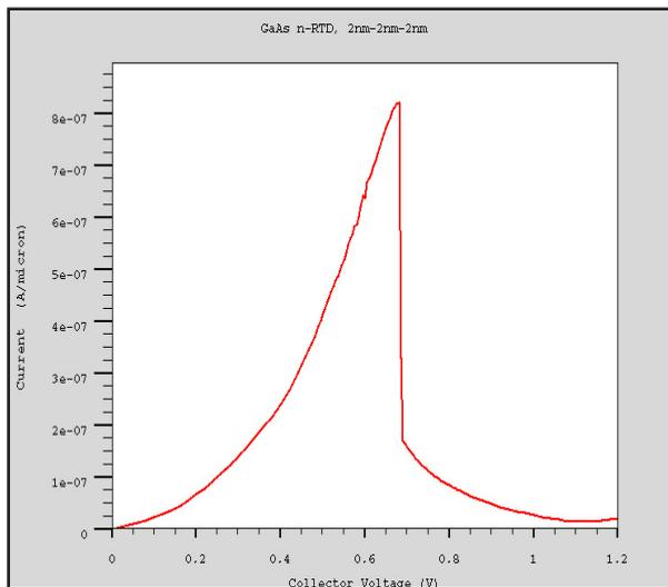
Figure 4. Current-voltage characteristics of n-type GaAs RTD.
