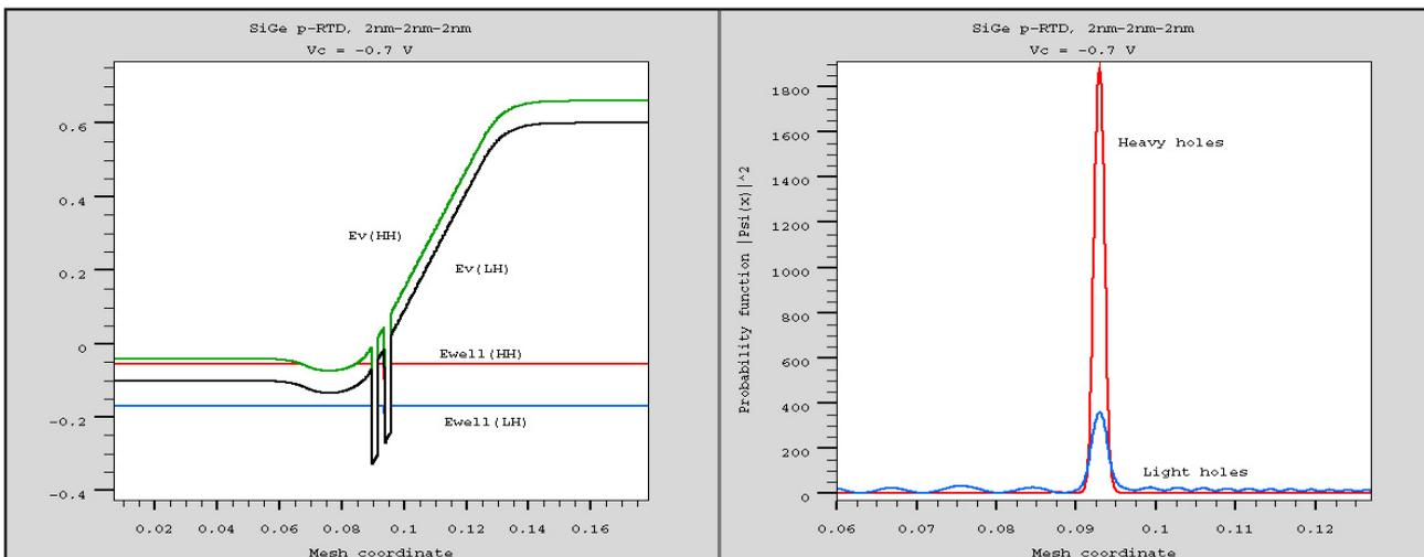
Figure 6. (Left panel) Valence band profile for heavy and light hole bands. Horizontal lines show highest bound state energies for the two bands. (Right panel) Probability function for the heavy and light hole states confined in the well.
