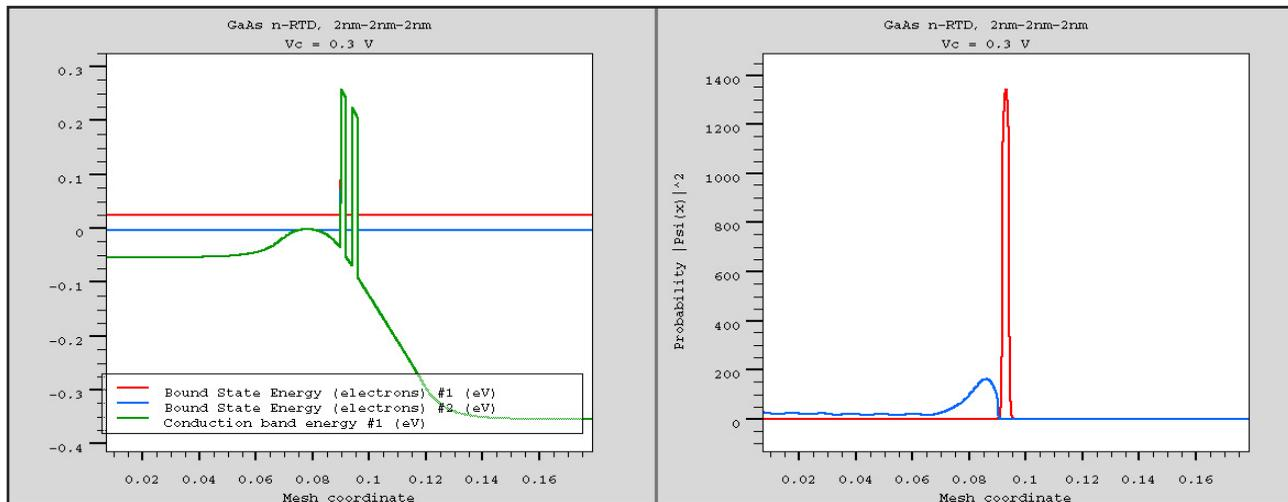
Figure 1. (Left panel) Conduction band profile at a bias of 0.3V. The horizontal lines show the eigen energies in the emitter (blue) and in the well (red). (Right panel) Probability functions, corresponding to the bound states in the emitter (blue) and the well (red).
