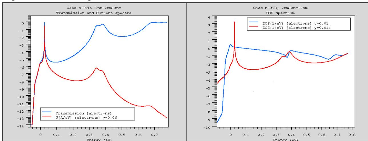
Figure 2. (Left panel) Spectrum of transmission (blue) and current density (red) at a bias of 0.3 V. (Right panel) Spectrum of the local density of states in the emitter (blue) and the well (red).
