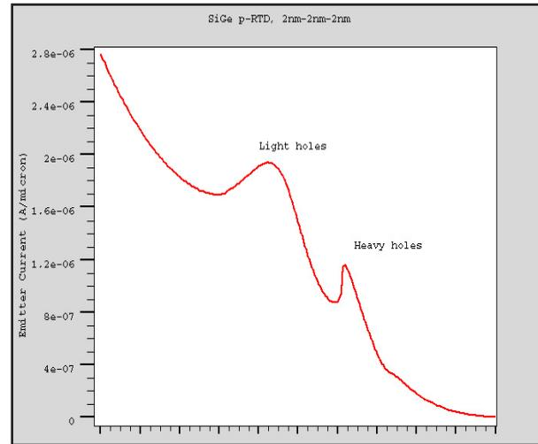
Figure 8. Current voltage characteristics of the SiGe p-type RTD. Multiple NDR regions correspond to different hole bands.
