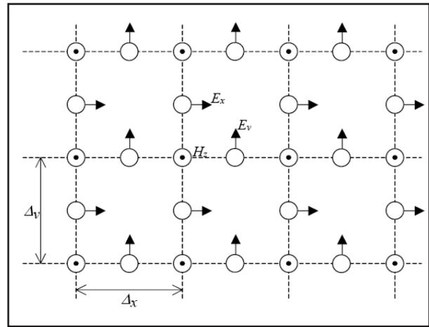
Figure 4. Two-dimensional FDTD calculation grid for TE-waves. The E- and H-evaluations are shifted half a step-size in time.
