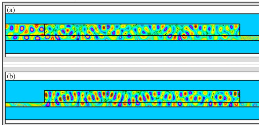
Figure 5. 2D FDTD simulated  $E_x$  profiles for TE mode of (a) Butt-coupled waveguide and (b) Evanescent-coupled waveguide.
