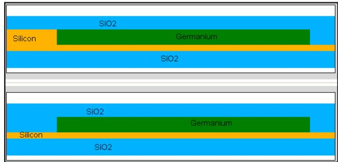
Figure 1. Schematic structure of waveguide PDs of (a) Butt-coupled type (b) Evanescent-coupled type.
