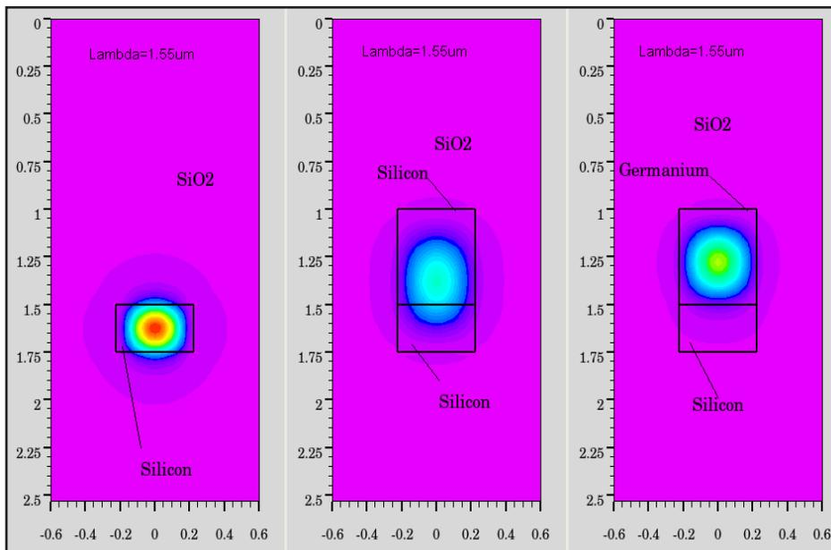
Figure 2 Fundamental optical mode-field profile of (a) a typical SOI high-index-contrast strip Si on waveguide for 1.55 $\mu\text{m}$  wavelength and (b) Si-Si SOI (c) Ge/Si on SOI photodiode.
