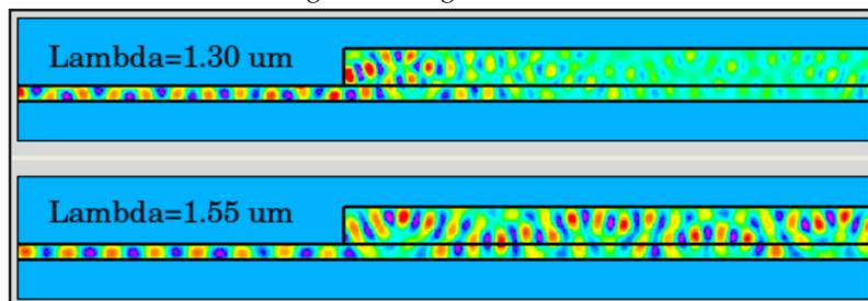
Figure 7 The Ex modes of the Evanscent-coupled waveguide at (a) 1.30um and (b) 1.55um of wavelength.
