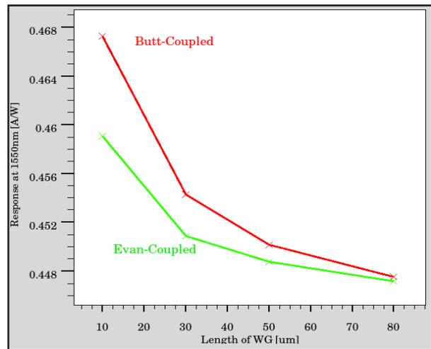
Figure 8. Inter responsivity at 1.55um as a function of Ge waveguide length for butt-coupled and evanescent-coupled photodiodes.
