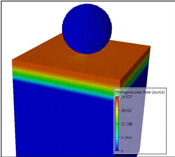
Figure 2: Three Dimensional Photogeneration Rate Under an Example Nano-particle.
