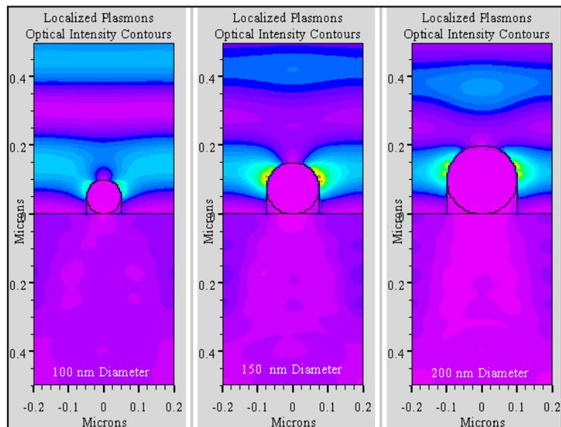
Figure 1: Optical Intensity Contours for Three Sizes of Nano-particle.
