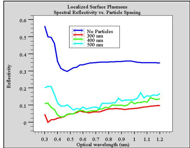
Figure 4: Comparison of Spectral Reflectivity vs. Nano-particle Spacing.
