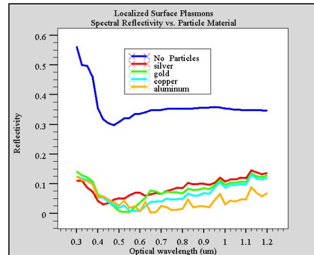
Figure 5: Comparison of spectral Reflectivity vs. Particle Composition.
