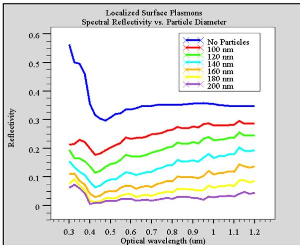
Figure 3: Comparison of Spectral Reflectivity vs. Nano-particle Diameter.
