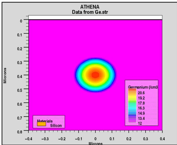
Figure 1. showing germanium impurity distribution for experiment 1 where the dopant is completely encapsulated within silicon.
