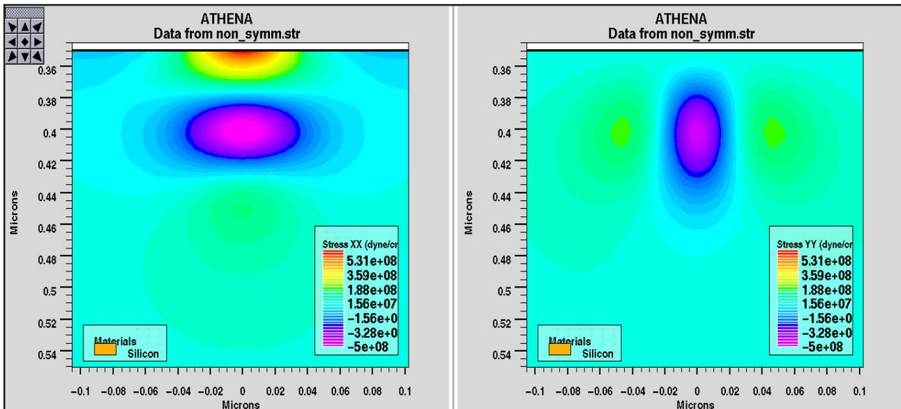
Figure 4 Resulting XX and YY direction stress fields as a result of the SiGe dot shown in Figure 3.
