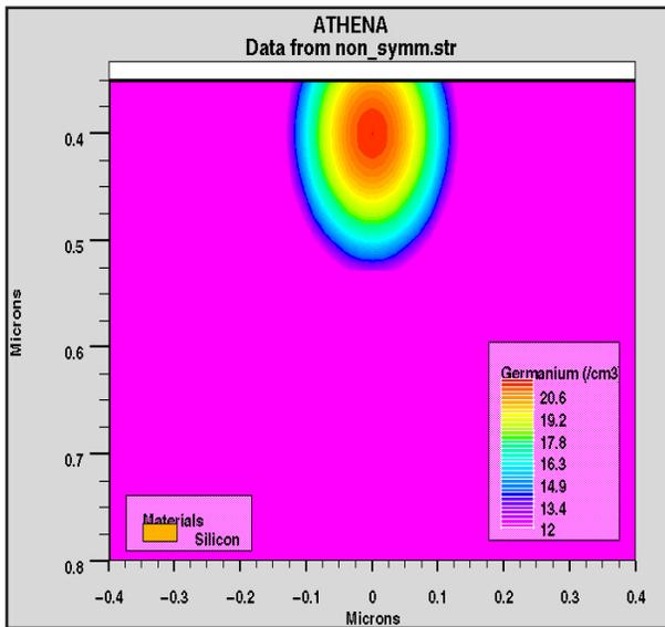
Figure 3 The test structure for experiment 2 showing the same SiGe “diffused dot” as in Figure 1, but with the surface of the structure etched away, leaving a non zero concentration of SiGe at the free surface.
