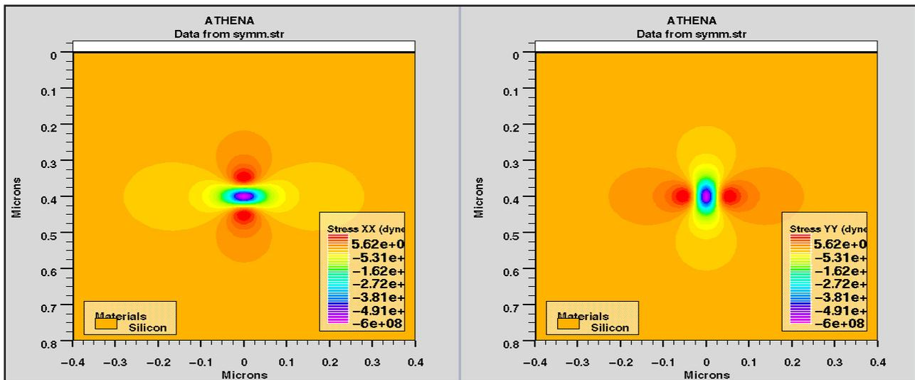
Figure 2. calculated stress fields in the XX and YY directions resulting from the buried SiGe dot shown in figure 1 .
