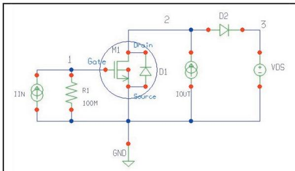
Figure 2. Test Circuit for Gate Charging
