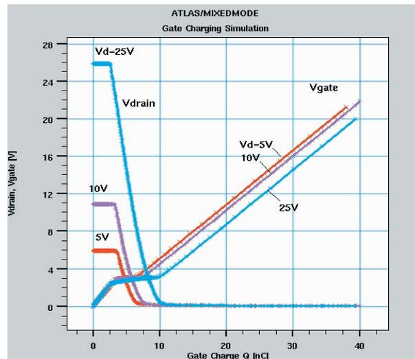
Figure 3. The waveform of the gate charging at gate current is 2mA
