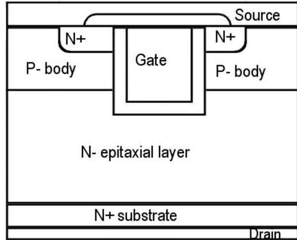
Figure 1. Typical UMOSFET Structure
