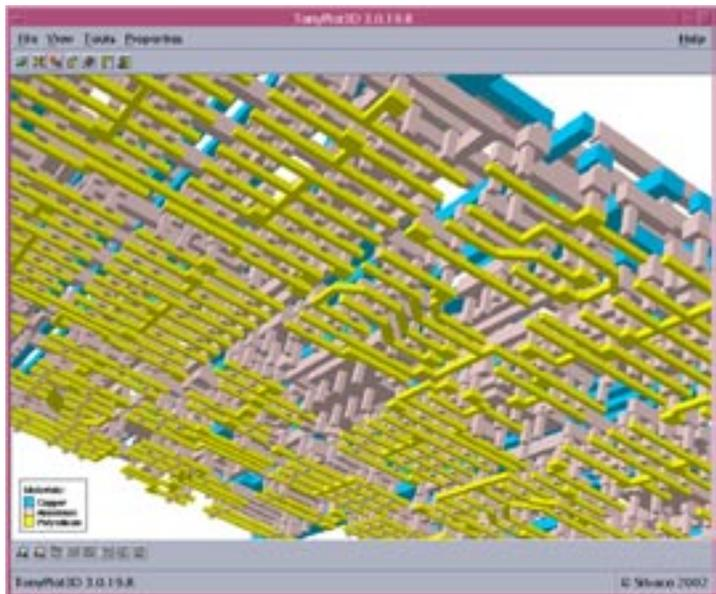
Figure 12. STELLAR generated 3D backend structure.
