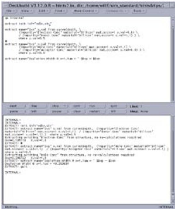
Figure 2. DeckBuild window that shows the runtime output of the EXTRACT commands.
