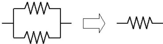
Figure 1. Parallel Resistor Reduction
