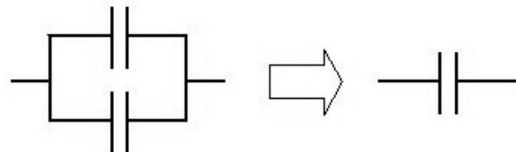
Figure 4. Parallel Capacitor Reduction
