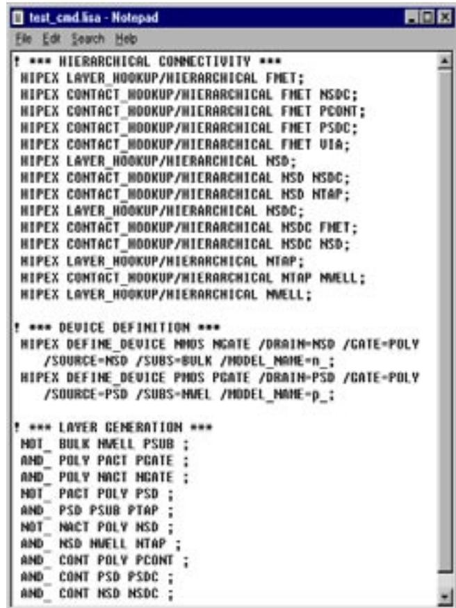
Figure 3. Fragment of technology file for *Hipex-NET*.
