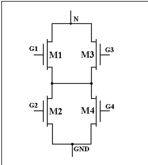
Figure 2. Series-parallel network of MOSFET transistors.
