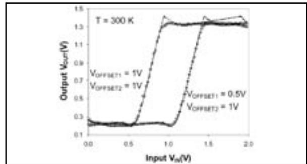
Figure 9. Characteristics of basic SET-CMOS hybrid neuron cell [5] (with  $C_G = C_{G2} = 0.04aF$ ,  $C_{TD} = C_{TS} = 0.02aF$ ,  $R_D = R_S = 1M\Omega$ ) as predicted by SIMON (symbol) and *SmartSpice* (solid & dotted line). Note:  $I_{bias}$  is taken to be ideal current source of 50nA for SIMON simulation and for *SmartSpice* simulation the MOS current source is designed in such a way that it can drive the same bias current through the SET.
