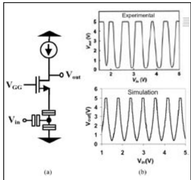
Figure10. (a) A schematic of the universal literal gate comprising a SET and a MOSFET [7]. (b) Comparison between measured and simulated  $V_{in}-V_{out}$  characteristics of the universal literal gate at  $T = 27K$ . The SET device parameters are  $C_G = 0.27aF$ ,  $C_{TD} = C_{TS} = 2.7aF$ ,  $R_D = R_S = 200k\Omega$  and MOS device parameters are  $W = 12\mu m$ ,  $L = 14\mu m$ ,  $t_{ox} = 90nm$ .  $V_{GG}$  is set to 1.08V and  $V_{out}$  is hard-limited at 5V.
