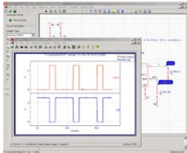
Figure 6. Simulation of RSFF Verilog-A module and results.
