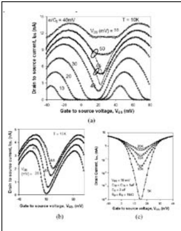
Figure 5: Verification of MIB model for (a) symmetric SET device with  $C_G = 2aF$ ,  $C_{TD} = C_{TS} = 1aF$  and  $R_D = R_S = 1M\Omega$ . Here symbols denote Monte Carlo simulation (SIMON) and solid line represents MIB LEVEL3 and dotted line represents MIB LEVEL2 (without  $|V_{DS}| > e/C_S$  correction). (b) asymmetric device with  $C_G = 2aF$ ,  $C_{TD} = 1.5aF$ ,  $C_{TS} = 0.5aF$  and  $R_D = 1M\Omega$  and  $R_S = 5M\Omega$  (c) effect of temperature on the device characteristics.
