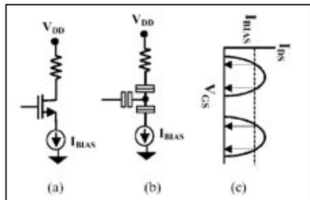
Figure 2. (a) A current bias MOSFET with a floating gate (b) corresponding SET prototype (c) Different possible value of the gate voltage for in (b) for a fixed current bias.
