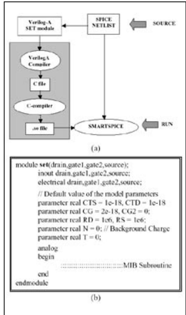
Figure 4. (a) Working principle of Verilog-A in SMARTSPICE (b) partial architecture of Verilog-A SET module.
