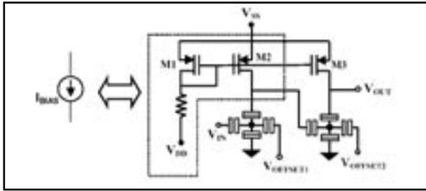
Figure 8. Basic structure for the realization of the activation function of a neuron as proposed by Goossens [8].
