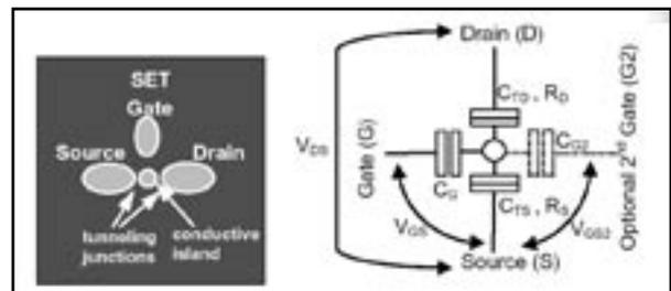
Figure 1. Schematic of a SET. Here  $C_G$  is the gate capacitance,  $C_{G2}$  is the optional second gate capacitance,  $C_{TD}$  and  $C_{TS}$  are the drain and source tunnel junction capacitances, respectively, and  $R_D$  and  $R_S$  are drain and source tunnel junction resistances, respectively.
