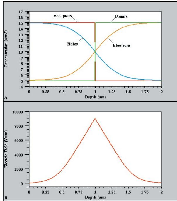
Figure 2. Dopant and carrier concentration profiles in neighboring p- and n-type silicon regions.
