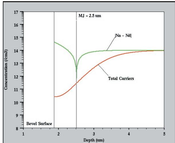
Figure 3d. Net doping and total carrier concentration profiles for simple gaussian PN junction after 1.875 microns of silicon has been removed.
