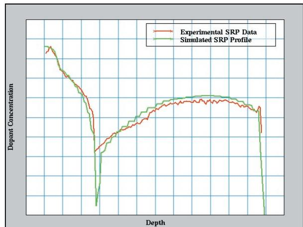
Figure 5. Comparison of simulated and measured SRP profiles for the source/drain region of a NMOS device.
