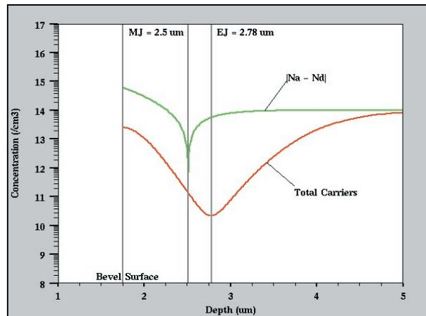
Figure 3b. Net doping and total carrier concentration profiles for simple gaussian PN junction after 1.75 microns of silicon has been removed.
