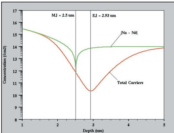
Figure 3a. Net doping and total carrier concentration profiles for simple gaussian PN junction.
