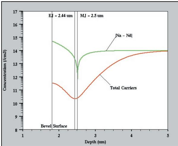
Figure 3c. Net doping and total carrier concentration profiles for simple gaussian PN junction after 1.8175 microns of silicon has been removed.
