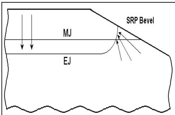
Figure 4. Two-dimensional cross section of beveled PN junction sample showing the qualitative effects of carrier spilling on a diffused p-layer in a lightly-doped n-type substrate.
