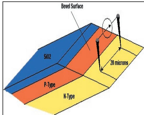
Figure 1. Schematic diagram of simple two-probe spreading resistance measurement system.
