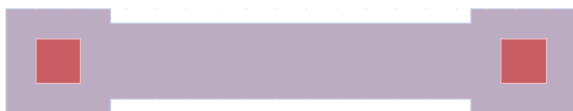
Figure 8. Resistor heads are parts of recognition layers: automatic calculation of head resistance.
