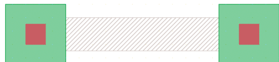
Figure 9. Resistor heads are not in recognition layers: head resistance should be prescribed.
