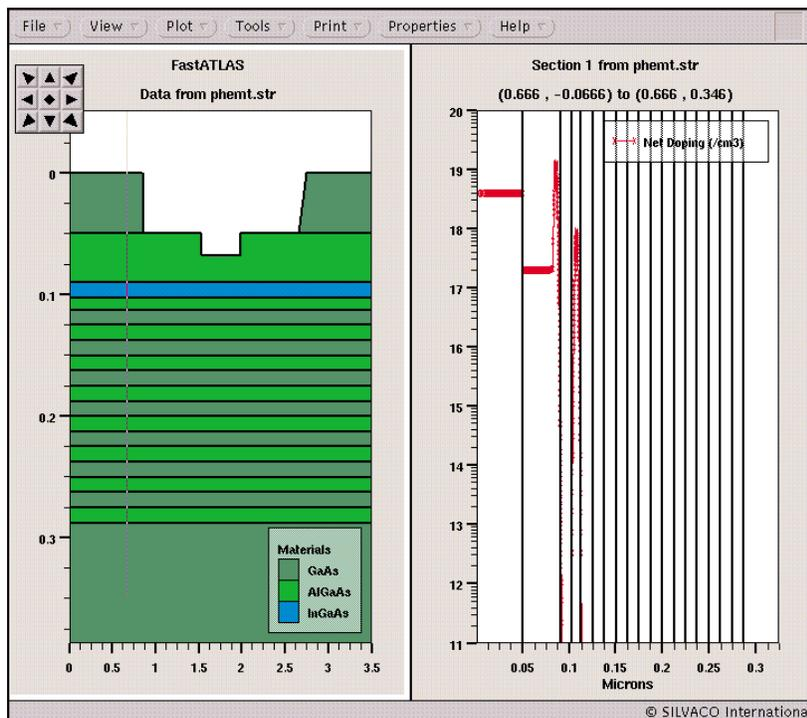
Figure 2. Two-dimensional structure of the initial PHEMT design and its net doping vertically through the source.
