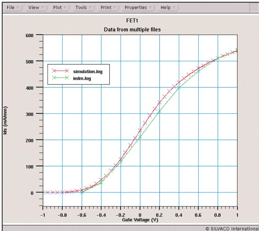
Figure 6. Comparison between the *FastBlaze* simulated drain current and measured data [1] as the gate voltage is swept from -1V to 1V.
