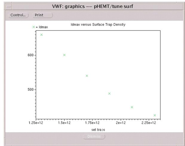
Figure 4. **FastBlaze** results showing effect of the surface trap density on the simulated maximum drain current.
