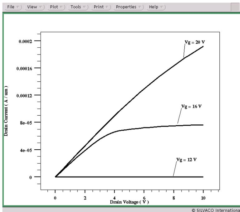
Figure 5: Drain Characteristics for UMOFET Structure for  $V_g=12\text{V}$ ,  $V_g=16\text{V}$ , and  $V_g=20\text{V}$  ( $\mu_{n0}=450 \text{ cm}^2/\text{Vs}$ ,  $VSATN=2.2 \times 10^7 \text{ cm/s}$ ,  $BETAN=1.2$ )
