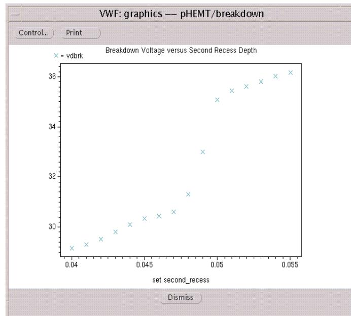
Figure 7. *FastBlaze* results showing the simulated variation of breakdown voltage with depth of the second recess.
