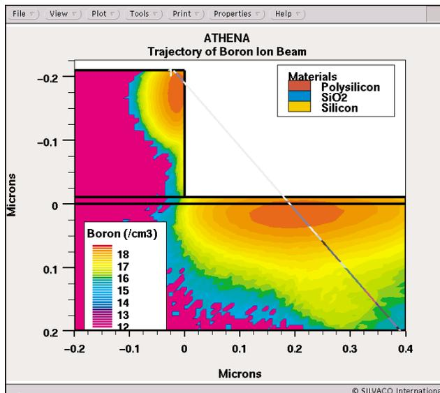
Figure 1. Showing device geometry effects. The Ion Beam passes through the top corner of the poly gate and into the silicon substrate below. In order to account for these effects, BCA also models the vacuum above the device.
