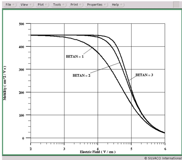
Figure 1: Mobility Versus Electric Field Generated Using Equation (1) for Several Values of BETAN ( $\mu_{n0}=450 \text{ cm}^2/\text{Vs}$ ,  $\text{VSATN}=2.2 \times 10^7 \text{ cm/s}$ )
