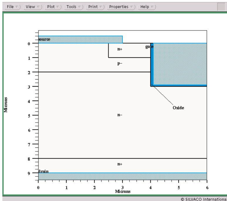
Figure 4: 4H-SiC UMOFET Structure Generated with ATLAS ( $n^+=5 \times 10^{19} \text{ cm}^{-3}$ ,  $n^-=2 \times 10^{15} \text{ cm}^{-3}$ ,  $p^-=2 \times 10^{17} \text{ cm}^{-3}$ )
