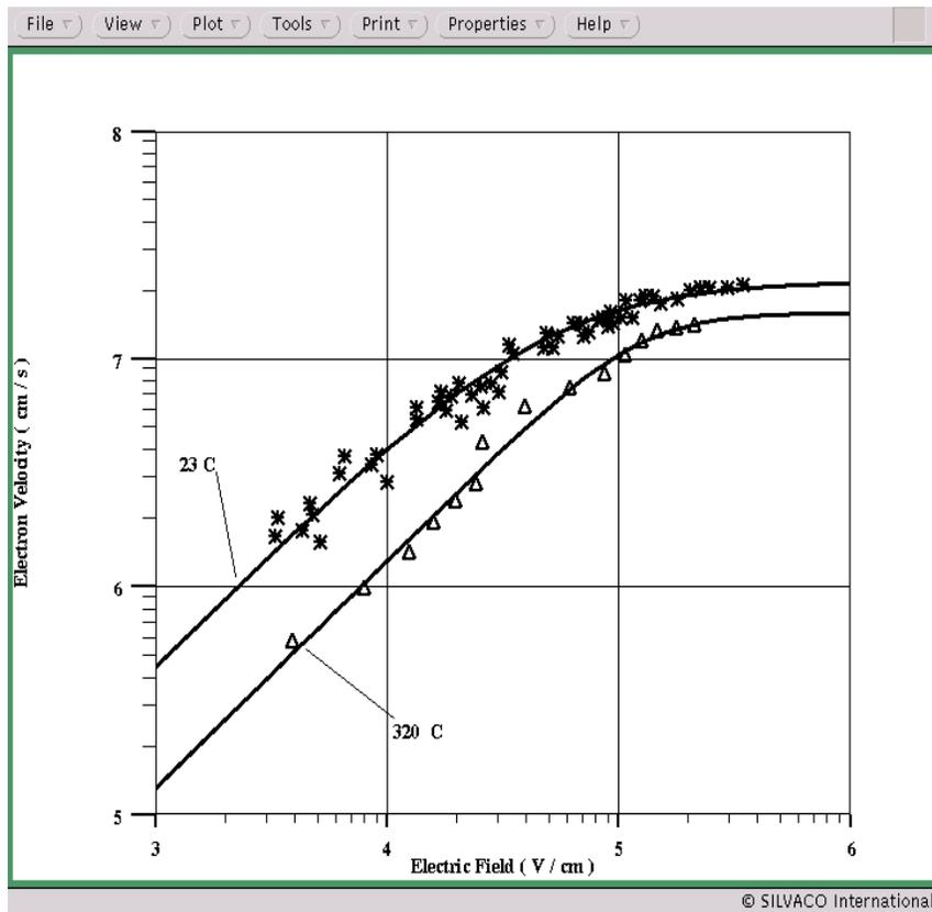
Figure 3: Velocity-Field Characteristics for (0001) 4H-SiC for Room Temperature and 320 °C, Simulated (solid lines), Experimental (symbols)
