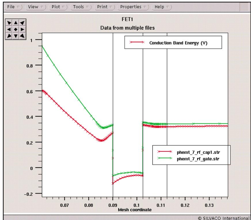
Figure 5. Conduction band profile under the recess of the PHEMT showing surface potential pinning.
