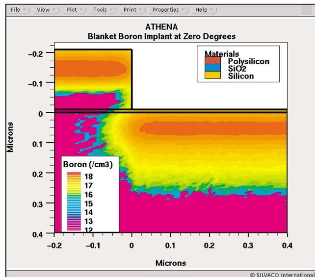
Figure 3. A zero degree tilt implant into the same structure for comparison.
