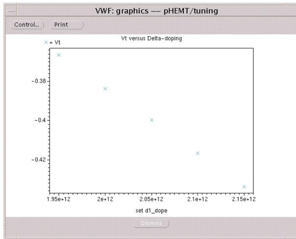
Figure 3. **FastBlaze** results showing the effect of delta layer doping on the threshold voltage.
