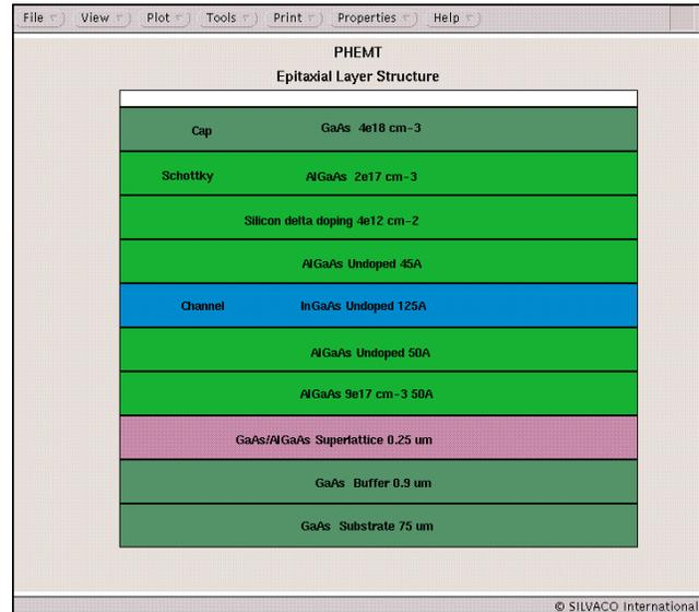
Figure 1. Layer structure of PHEMT[1] used in the *FastBlaze* simulation.
