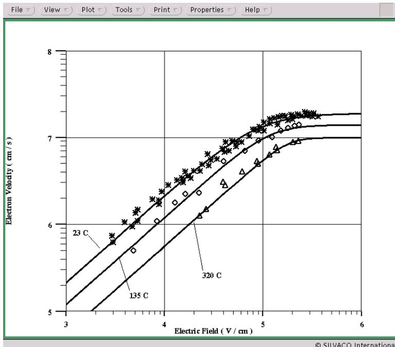
Figure 2: Velocity-Field Characteristics for (0001) 6H-SiC for 23 °C, 135 °C, and 320 °C, Simulated (solid lines), Experimental (symbols).
