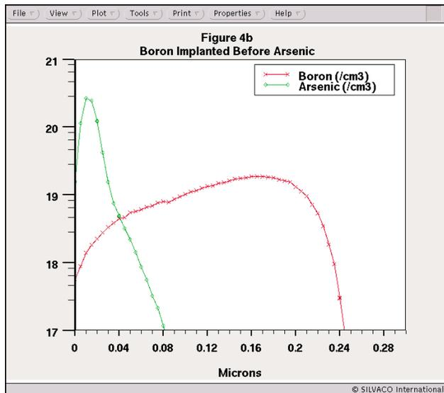
Figure 4. Comparison between two identical process flows, but where the order of two identical implants is switched. In the first profile (Figure 4a), the arsenic is implanted first, the surface is amorphised and little channelling occurs in the following boron implant. When the implant order is switched, significant channelling of boron occurs (Figure 4b).
