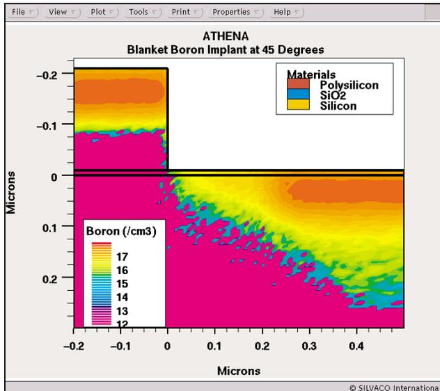
Figure 2. The same implant conditions as Figure 1 but a blanket implant instead of a pencil beam. Channelling and shadowing effects are clearly demonstrated. Note the difference in implant depth between the polysilicon and the crystalline substrate.
