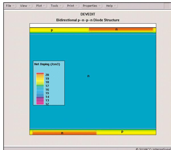
Figure 3. Bidirectional *p-n-p-n* diode switch structure created in *DevEdit*.
