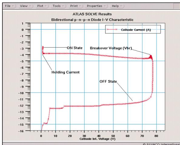
Figure 4. Simulated I-V characteristic of p-n-p-n diode from *ATLAS*.
