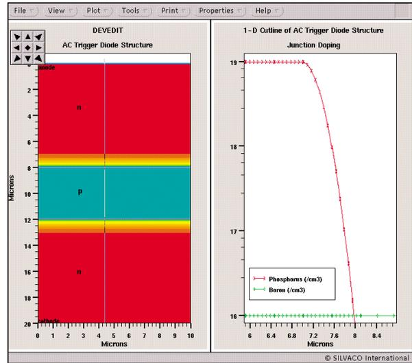
Figure 1. AC trigger diode structure created in *DevEdit*.
