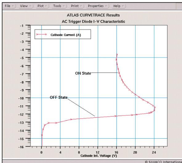
Figure 2. Simulated I-V characteristic of AC trigger diode structure from *ATLAS* Curvetrace routine.
