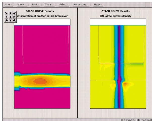
Figure 5. Simulated impact ionization rate at breakdown and total current density after device turn-on.
