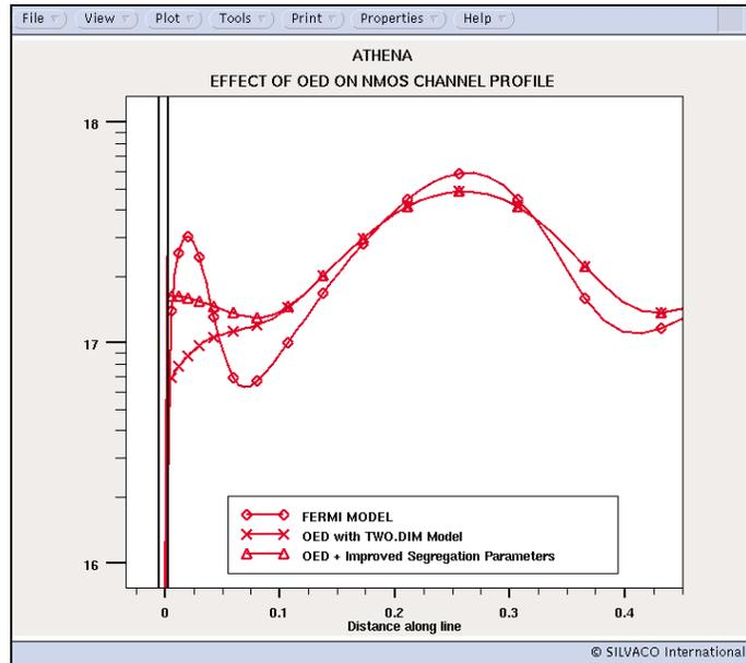
Figure 1. Comparison of FERMI and TWO.DIM models for NMOS channel implants and 8nm gate oxidation.
