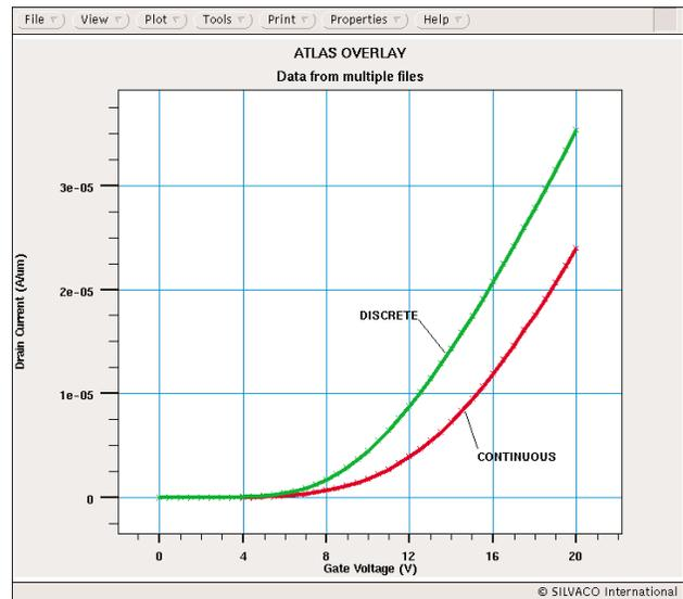
Figure 3 Id-Vg Characteristics of the TFT transistor showing the effect of the DISCRETE and CONTINUOUS models in the linear regime.
