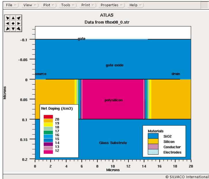
Figure 1. Geometry and doping profile of the Polysilicon TFT to be simulated.
