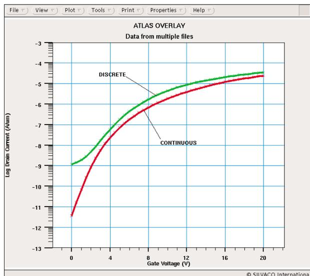
Figure 4 Log(Id)-Vg Characteristics of the TFT transistor showing the effect of the DISCRETE and CONTINUOUS models in the subthreshold regime.
