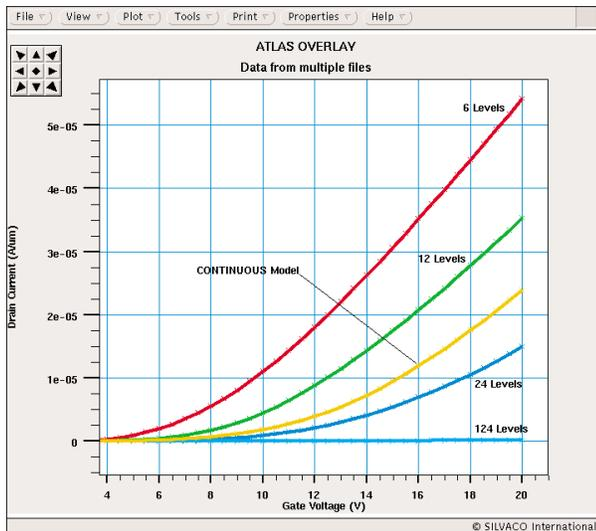
Figure 5. The number of trap levels in the DISCRETE model is shown to significantly influence the Id-Vg result. The CONTINUOUS model does not have this drawback.
