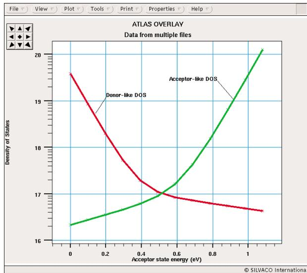
Figure 2 Density of States Profile for the Polysilicon TFT for both the donor and acceptor like traps..
