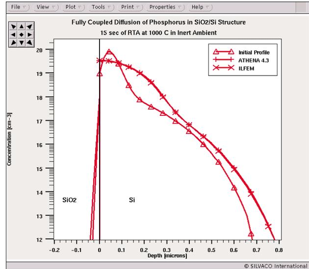
Figure 2. Fully coupled phosphorus diffusion using ILFEM.
