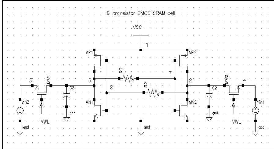
Figure 1. Schematic Diagram of a Six Transistor SRAM Cell
