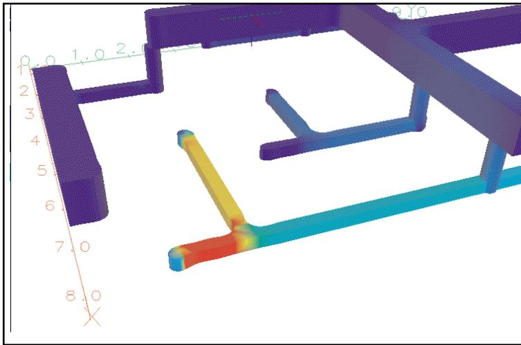
Figure 3. Current density in the interconnect. Note the lithographic geometry.
