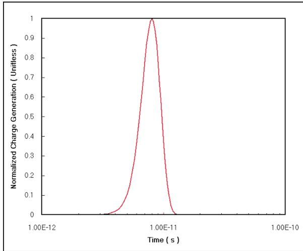
Figure 3. Single Event Upset Normalized Charge Generation Versus Time
