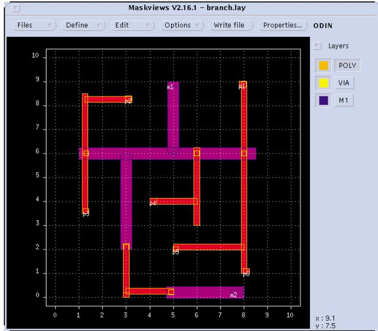
Figure 1. Layout of net within a cell. Combining this geometry with process information allows *Clever* to create a 3D structure of the conductors.
