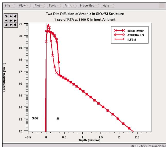
Figure 3. Defect enhanced diffusion of arsenic using ILFEM enhanced.
