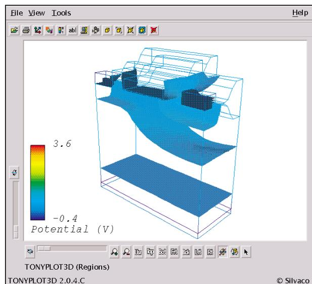
Figure 7. Potential Isosurfaces (a) Before SEU Strike (b) During SEU Strike When Electron-Hole Pair Generation is Near a Maximum.
