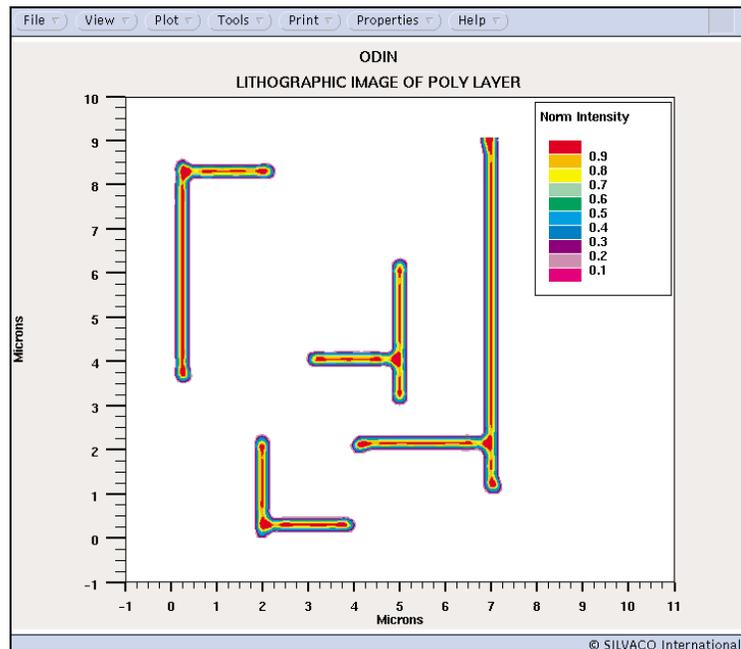
Figure 4. Optical image of the POLY layer from the layout in Figure 1.
