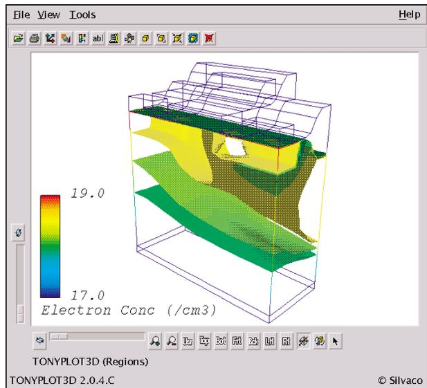
Figure 6. Electron Concentration Isosurfaces (a) Before SEU Strike (b) During SEU Strike When Electron-Hole Pair Generation is Near a Maximum
