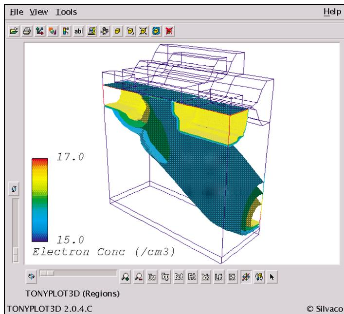
Figure 4. Three-Dimensional NMOSFET Structure Showing Location of Single Event Upset Strike.
