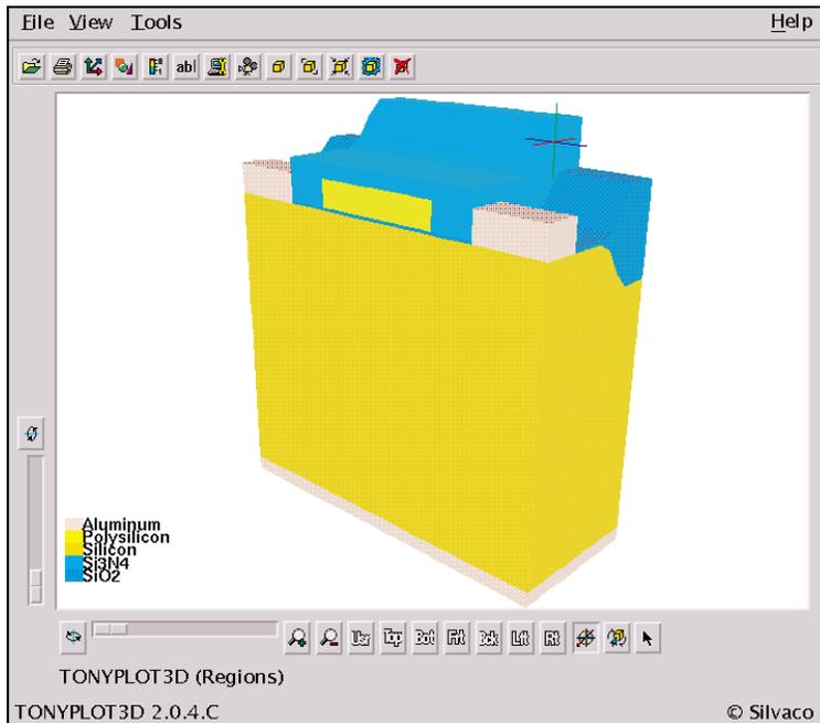
Figure 2. Three-Dimensional NMOSFET Structure Created With *DevEdit3D*.
