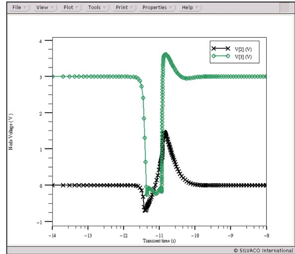
Figure 5. Internal SRAM storage Node Voltage Versus Time.
