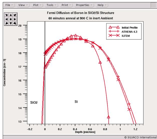
Figure 1. Boron anneal using ILFEM and ATHENA.
