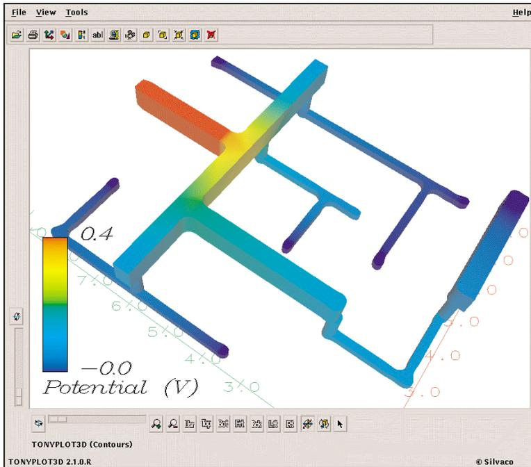
Figure 2. Potential distribution within the interconnect of the net.
