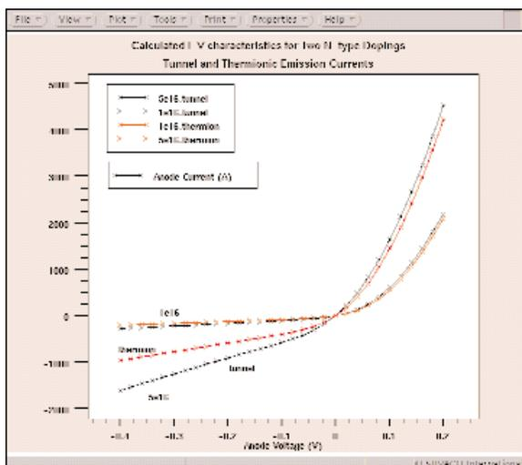
Figure 2: Calculated I-V characteristics of an n-GaAs / n-AlGaAs diode. Units of current are Amps/cm<sup>2</sup>.
