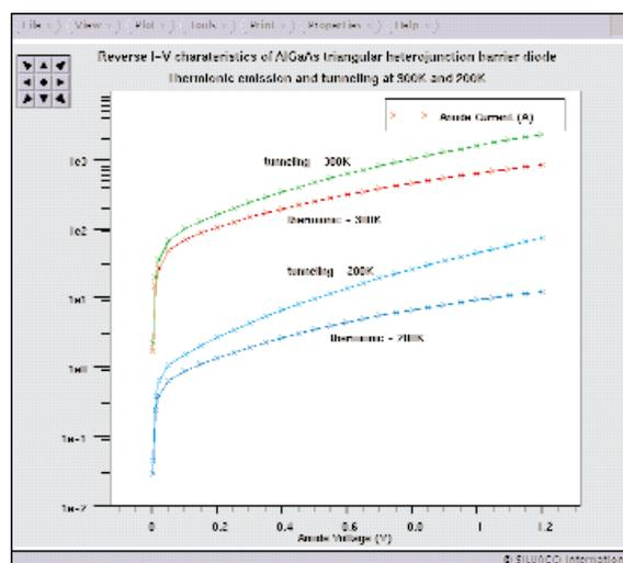
Figure 5: Reverse Bias I-V characteristics at 300K and 200K of thermionic emission and tunneling currents for a graded isotype GaAs-AlGaAs barrier.
