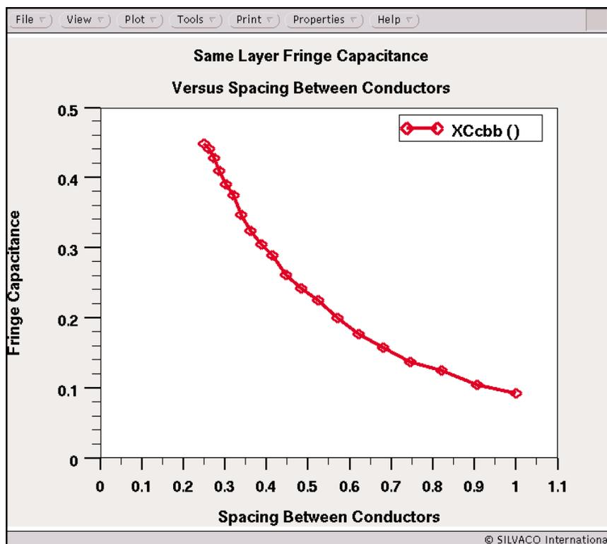
Figure 9. Same Layer Fringing Capacitance versus Line Spacing .
