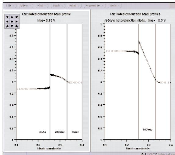
Figure 3: Calculated conduction band profiles of a GaAs - AlGaAs - GaAs diode at bias of a) 0.15 V and b) -0.5V.
