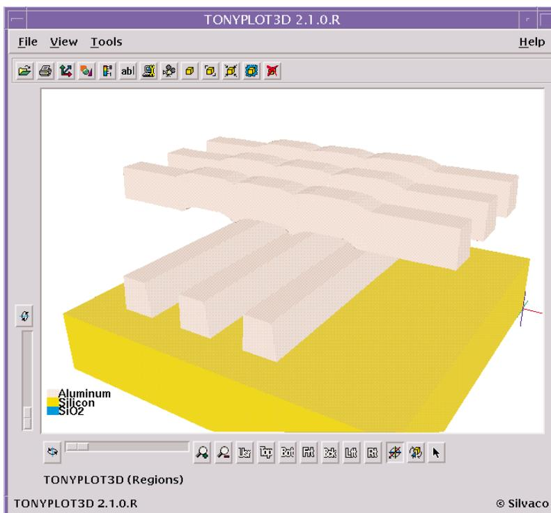
Figure 1. An example 3D test structure created by **EXACT** for capacitance coefficient calculations.
