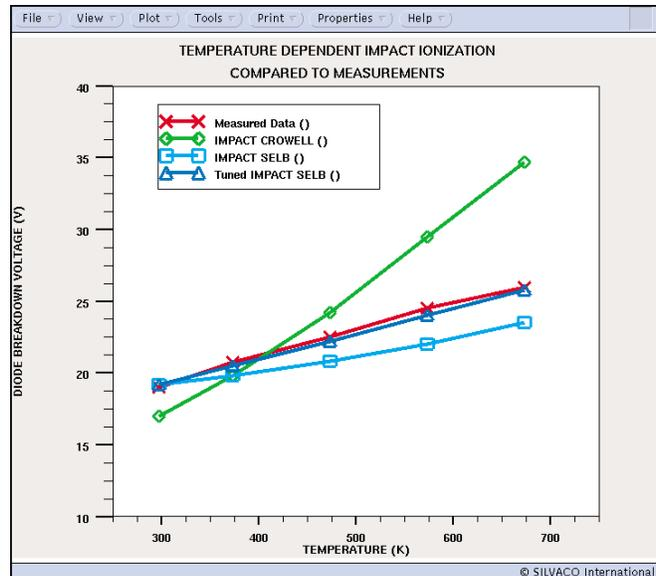
Figure 1. Comparison of default and tuned models in *ATLAS* to measured data for breakdown voltage vs. temperature.
