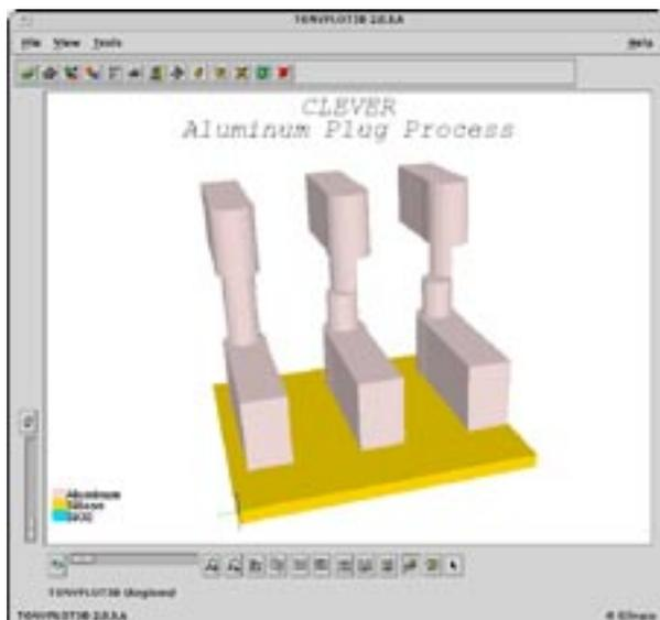
Figure 2. Geometry of Al plug process with from left to right, zero, 0.1  $\mu\text{m}$  and 0.15  $\mu\text{m}$  misalignment of the metal 2 layer.
