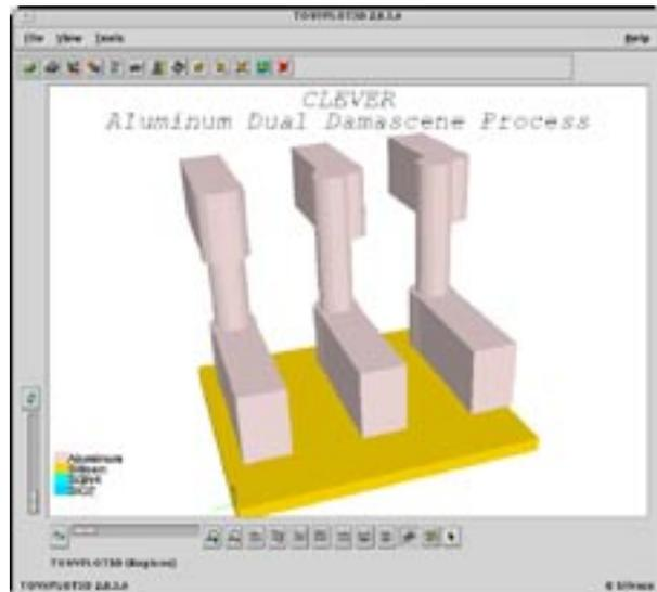
Figure 4. As figure 2, but for Al dual-damascene process. Note the increase in contact area with misalignment.
