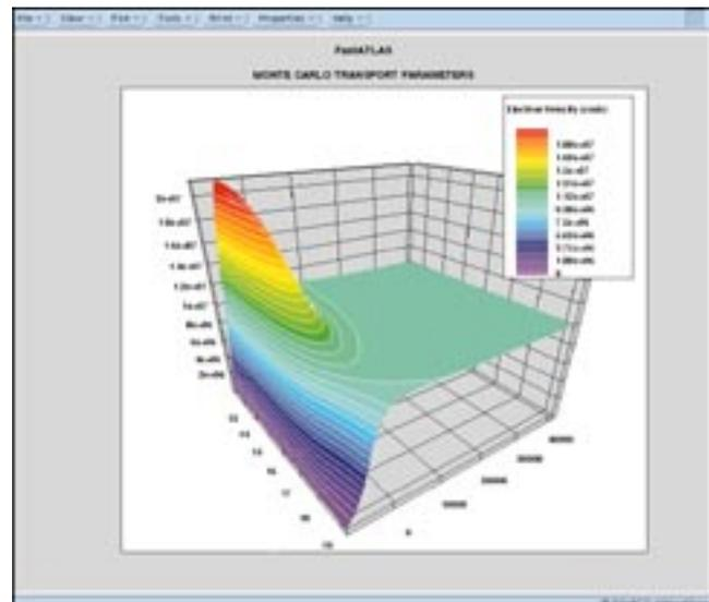
Figure 1. Monte Carlo generated electron velocity as a function of doping and field. This data is used by *FastBlaze* for accurate carrier transport simulation.
