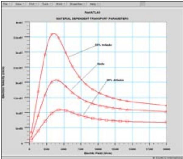
Figure 2. Velocity-field characteristics for various III-V materials.
