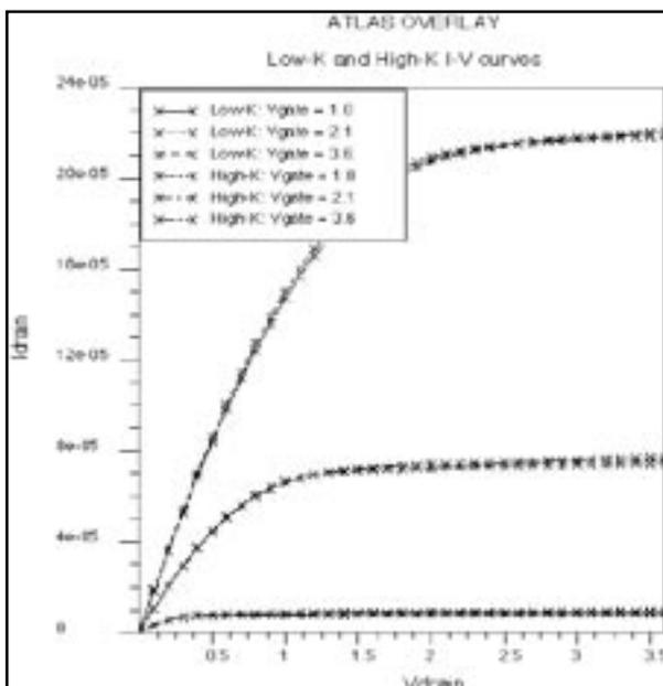
Figure 2.  $I_D$ - $V_{DS}$  comparison of high-K gate dielectrics versus conventional processing. The high K material allows equal drive current with a thicker dielectric.
