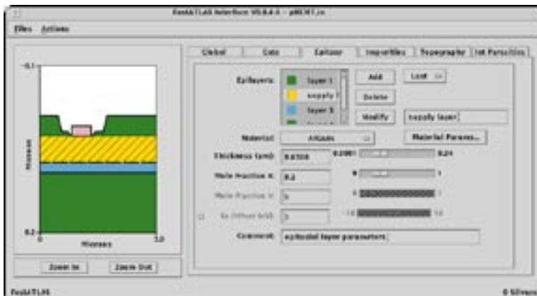
Figure 6. The **FastBlaze** GUI is called from **DeckBuild** and allows easy definition of complex III-V FET structures for FastBlaze.
