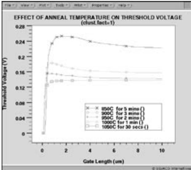
Figure 2. Showing the effect of anneal conditions on the threshold voltage of a MOSFET.
