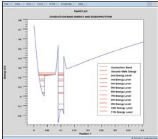
Figure 3. Quantized states in a pHEMT.
