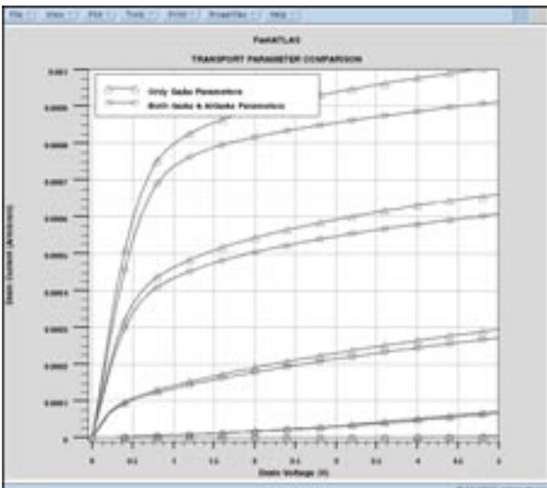
Figure 4. Comparison of HEMT Id-Vd using correct multi-layer transport models. The AlGaAs transport parameters are derived from Mocasin.
