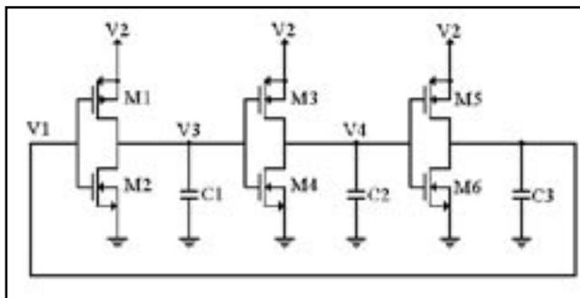
Figure 1. Schematic Diagram of Three Stage CMOS Ring Oscillator Used in MixedMode Simulation.
