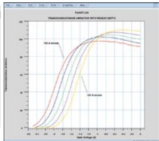
Figure 7. Experimentation using **FastBlaze** is quick and simple. Here the transconductance is shown as a function of recess depth.
