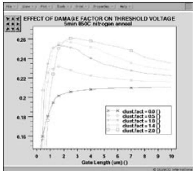
Figure 1. Showing the effect of changing the *CLUST.FACT* damage factor in *ATHENA*.
