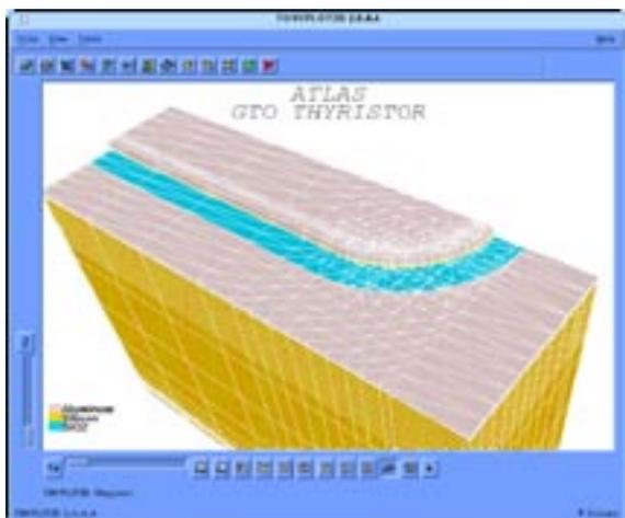
Figure 2. GTO thyristor geometry. This device can only be simulated correctly in 3D.
