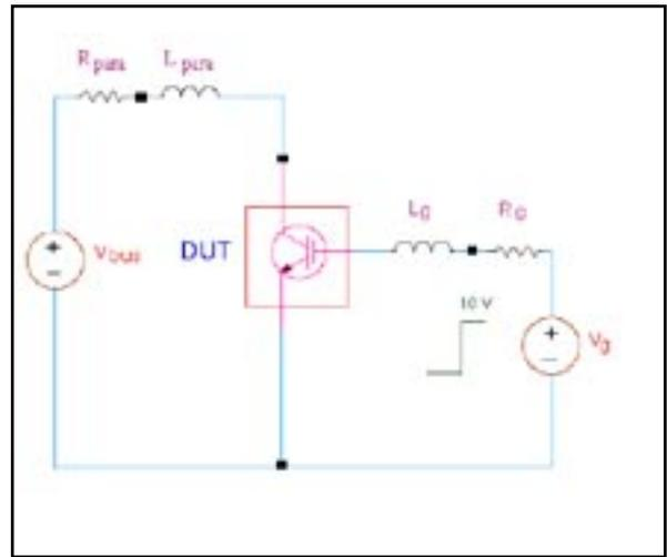
Figure 4. Test circuit used for short-circuit switching study.
