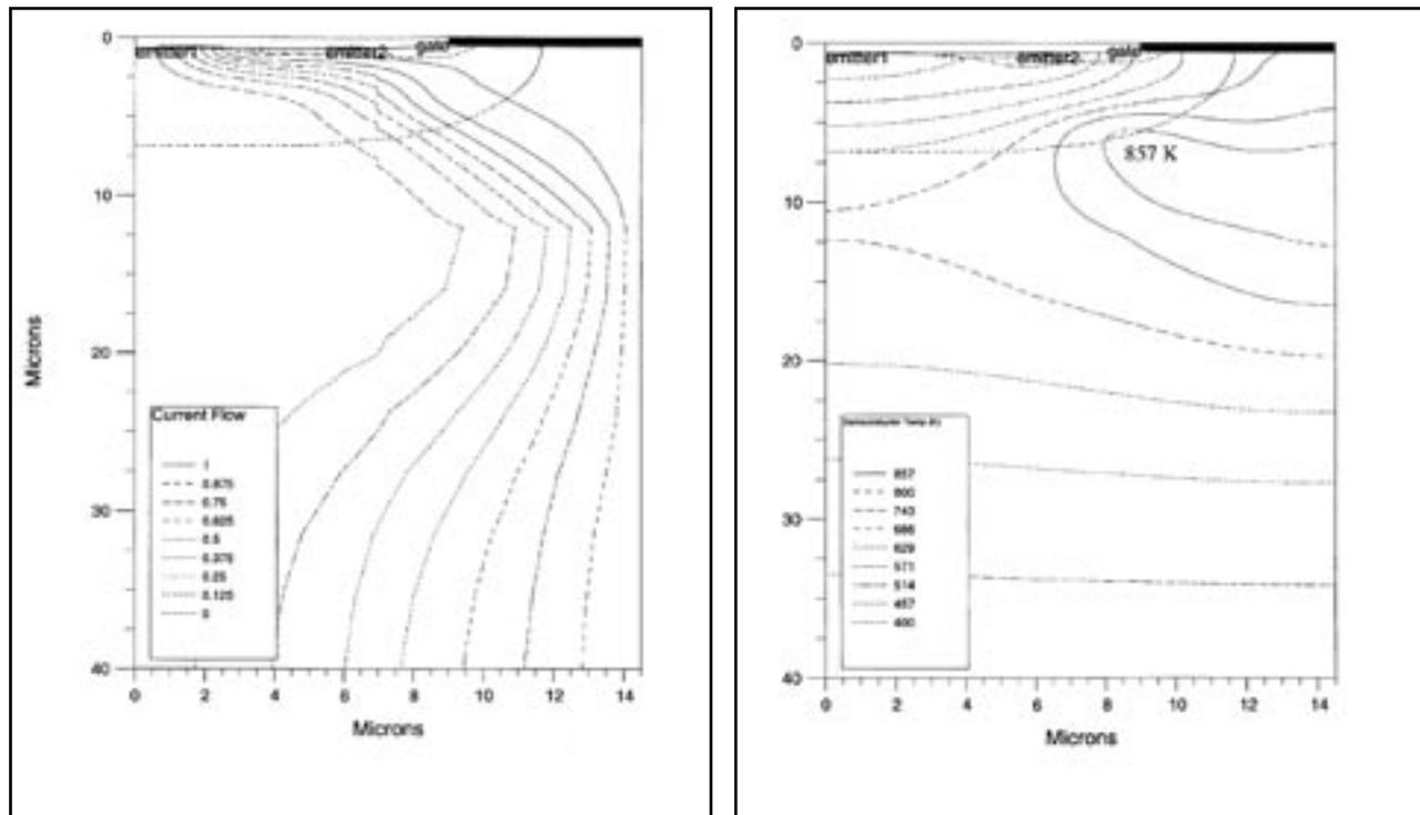
Figure 6. (left) Current flowlines, and (right) temperature distribution within the device at short circuit failure.
