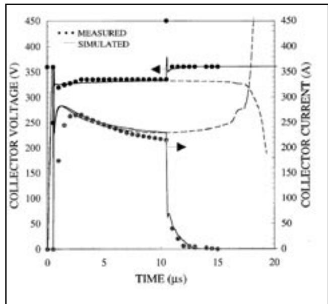
Figure 5. Measured and simulated short circuit performance of IGBT.
