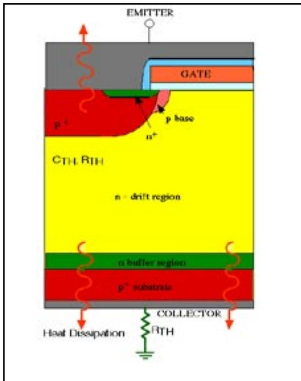
Figure 2. Two-dimensional representation of Insulated Gate Bipolar Transistor along with thermal resistance at collector electrode.
