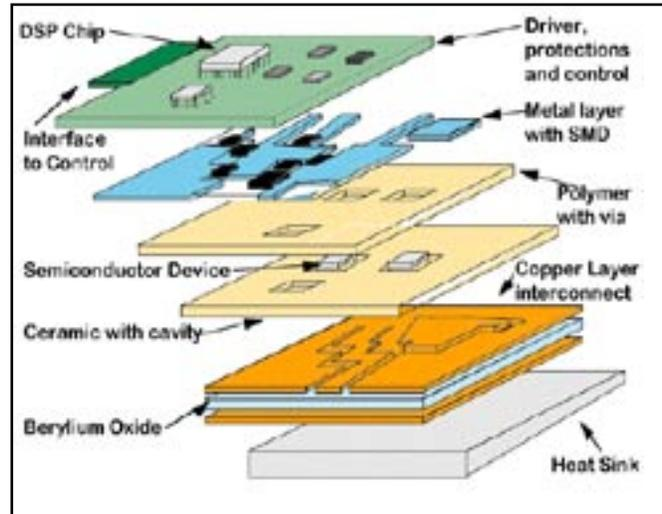
Figure 1. Components of a Power Device Module Packaging.
