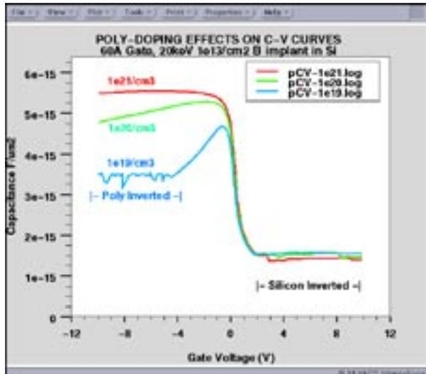
Figure 1. C-V curves showing the effect of different doping concentrations in the poly gate.
