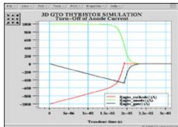
Figure 5. Currents in the GTO thyristor during turn-off through external circuit.
