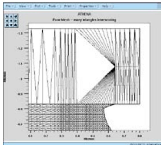
Figure 2. Mesh triangles sharing a common vertex. Due to discontinuous size mesh between materials, the mesh in the top layer is distorted.
