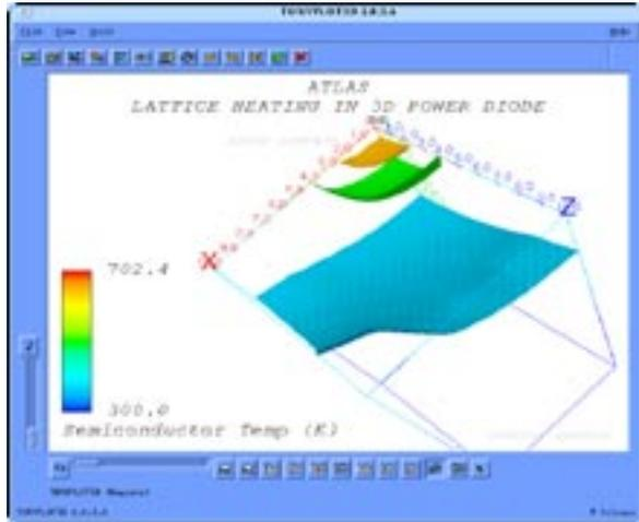
Figure 3. Isosurfaces of temperature in a power diode with current crowding into the anode.
