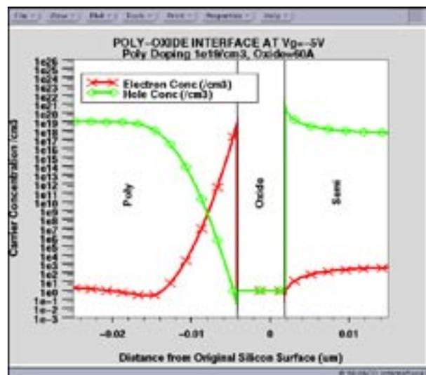
Figure 2. Carrier concentrations at the Oxide-Polysilicon interface showing inversion in the polysilicon gate.
