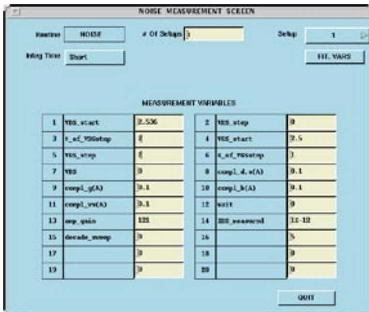
Figure 1. Noise Measurement Routine Setup Screen.
