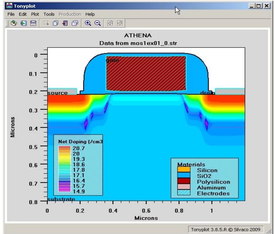
Figure 2.6. Process Simulated Structure Showing Net Doping.
