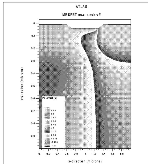
Figure 3. Potential contour - MESFET near pinch off.
