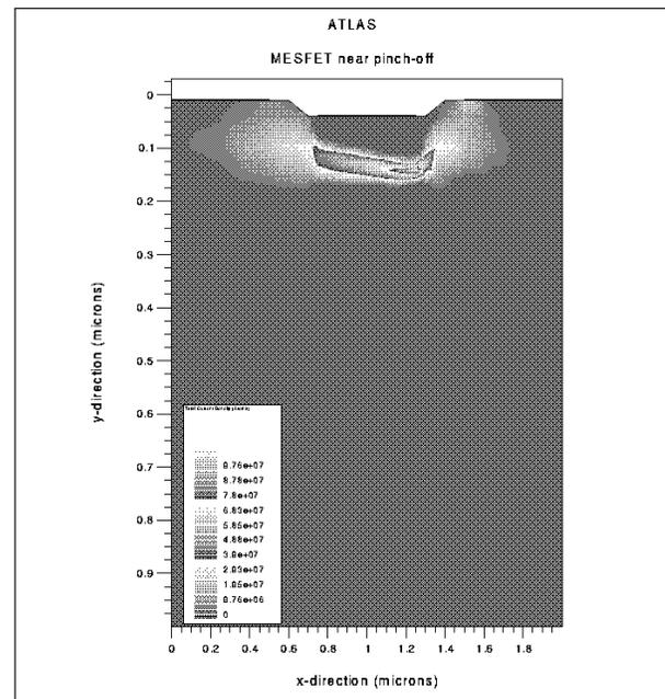
Figure 4. Total current density showing channel bounded by p-type doping layer.
