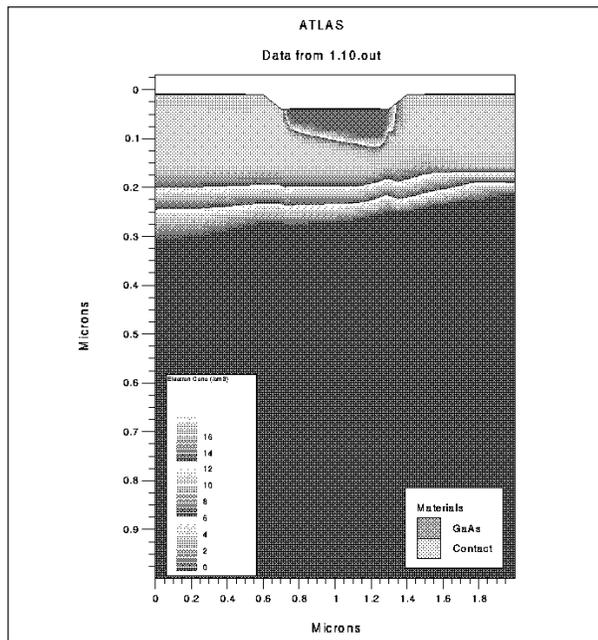
Figure 2. Electron concentration showing gate depletion region.
