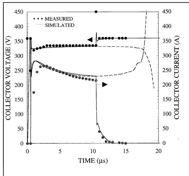
Figure 5. Measured and simulated short circuit performance of IGBT.
