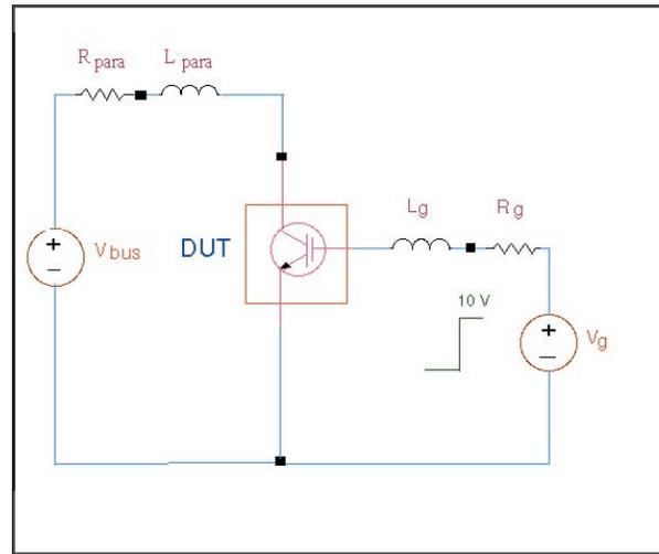
Figure 4. Test circuit used for short-circuit switching study.
