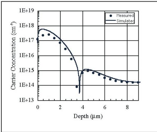
Figure 3. Measured and simulated doping profile of the p-base of IGBT.
