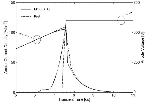
Fig.8 Turn-off waveforms of 1.2kV MOS-GTO and IGBT for a commutated anode current density of about 100A/cm<sup>2</sup>.
