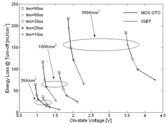
Fig.11 Comparison of trade-off curves for 4.5kV devices at different commutated anode current density  $J_A$ .
