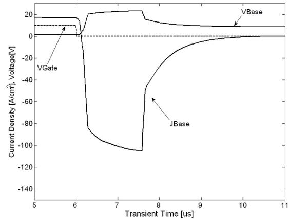
Fig.9 Base current density, base voltage and gate voltage progress during the turn off of 1.2kV MOS-GTO .
