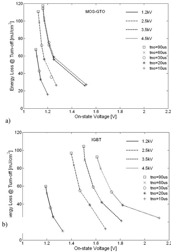
Fig.10 Trade-off curves of a) MOS-GTO and b) IGBT devices with different blocking voltage at  $J_A=100A/cm^2$ . The curves are obtained for different value of N-drift region lifetime with  $t_{p0}=t_{n0}/3$ .
