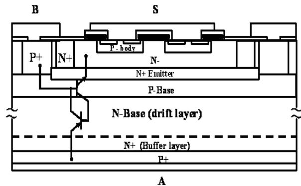
Fig.1. Schematic of the elementary cell of the proposed device.
