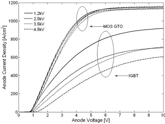
Fig.7. Comparison between the on state characteristics of MOS-GTO and IGBT devices having different blocking voltage.
