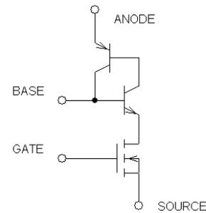
Fig.2. Equivalent circuit of the proposed device.
