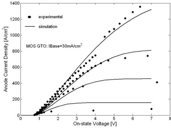
Fig.3. Experimental and simulated forward characteristics of 1.2kV device varying the gate voltage. For the simulated device the N-drift region lifetimes are fixed to  $\tau_{no}=10\mu s$  and  $\tau_{po}=3\mu s$ .
