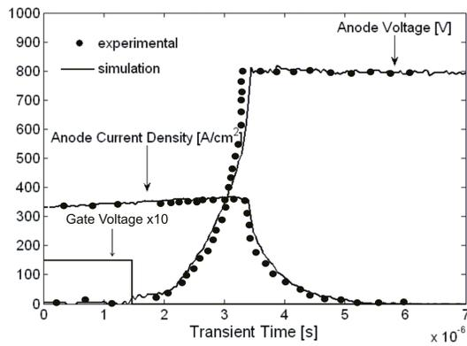
Fig.4. Experimental and simulated turn-off waveforms of 1.2kV MOS-GTO.
