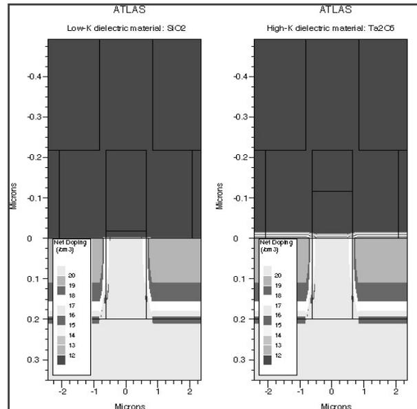
Figure 1. Device structures constructed in DEVEDIT for an NMOSFET comparing  $\text{SiO}_2$  and  $\text{Ta}_2\text{O}_5$  gate dielectric materials.
