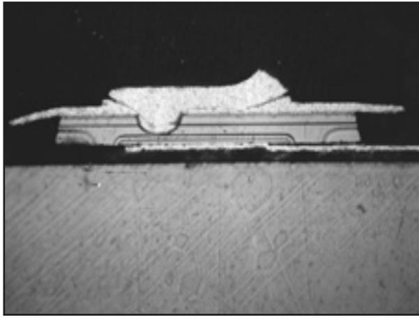
Figure 3. A photograph of a cross section of a short circuited MESA diode as a result of a pinhole.
