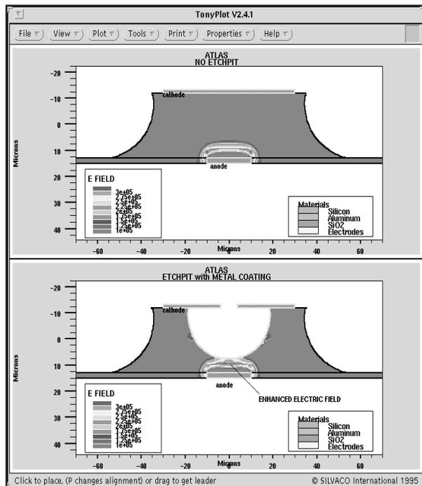
Figure 2. Electric field distribution in structures with and without etchpits.
