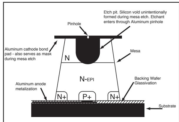
Figure 1. Schematic of Diode Array Mesa with etchpit defect
