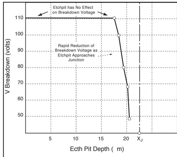
Figure 4. Breakdown voltage as a function of Etchpit Depth.
