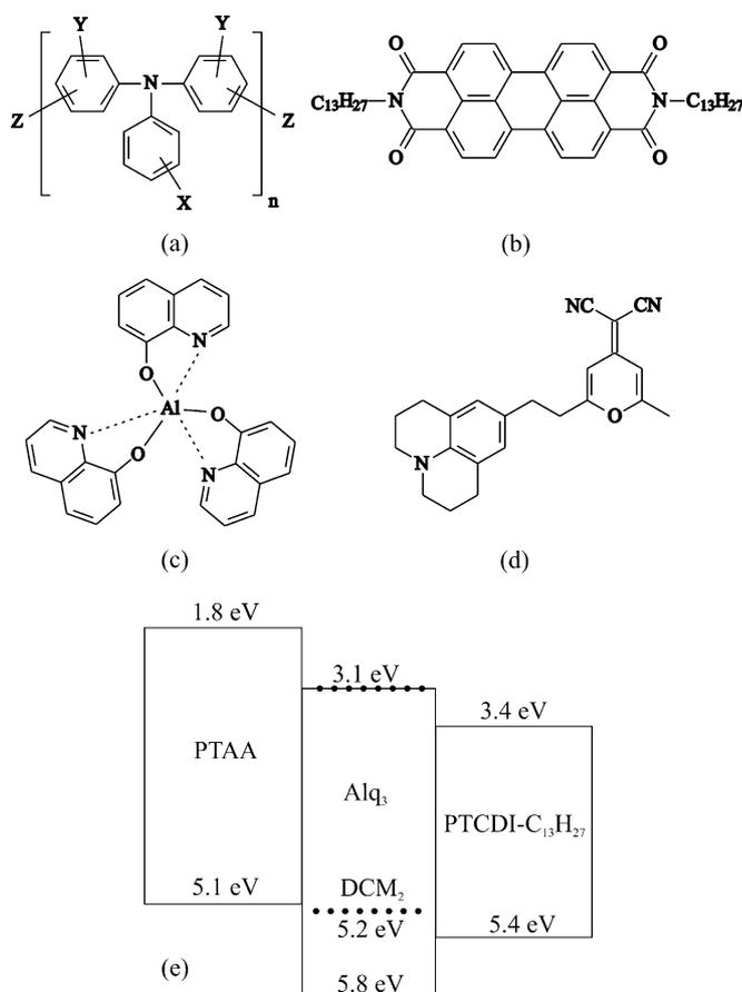
**Figure 4.** Molecular structure of the organic materials used to fabricate the light-emitting device: a) PTAA, b) PTCDI-C<sub>13</sub>H<sub>27</sub>, c) Alq<sub>3</sub>, and d) DCM<sub>2</sub>. e) Energy level diagram for these materials. The dotted lines indicate the highest occupied molecular orbital (HOMO) and the lowest unoccupied molecular orbital (LUMO) positions of DCM<sub>2</sub>.
