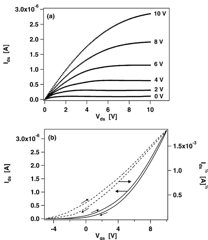
**Figure 6.** Electrical characteristics of a top-contact transistor comprising PTAA/Alq<sub>3</sub>:DCM<sub>2</sub>/PTCDI-C<sub>13</sub>H<sub>27</sub> as the organic layers ( $W/L = 2000/50$ ). a) Output characteristics for various gate voltages, and b) transfer characteristics of the same transistor. A saturation mobility of 0.08 cm<sup>2</sup> V<sup>-1</sup> s<sup>-1</sup> and a threshold voltage of ca. 0 V are extracted for this device.
