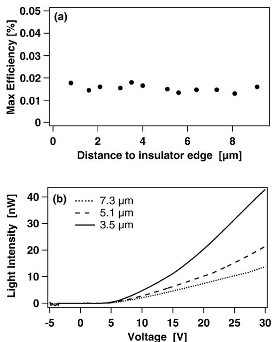
**Figure 12.** a) The maximum external quantum efficiency as a function of the distance from the insulator edge. The maximum external quantum efficiency is constant irrespective of the distance. b) Light intensity versus applied voltage of three different devices for which the top-contact displacement with respect to the insulator edge is 7.3  $\mu\text{m}$  (dotted lines), 5.1  $\mu\text{m}$  (dashed lines), and 3.5  $\mu\text{m}$  (solid lines).
