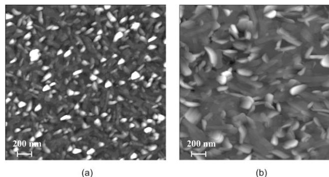
**Figure 7.** 2 μm × 2 μm atomic force microscopy surface scans of 50 nm thick PTCDI-C<sub>13</sub>H<sub>27</sub> layers on top of a) PTAA and b) PTAA/Alq<sub>3</sub>:DCM<sub>2</sub>. A higher surface roughness is measured for PTAA/Alq<sub>3</sub>:DCM<sub>2</sub>. The rms roughness is 10.7 nm for PTCDI-C<sub>13</sub>H<sub>27</sub> on PTAA/Alq<sub>3</sub>:DCM<sub>2</sub> versus 6.7 nm for PTCDI-C<sub>13</sub>H<sub>27</sub> grown on PTAA.
