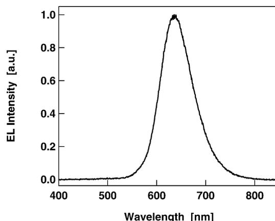
**Figure 9.** Normalized electroluminescence spectrum of the light-emitting diode with field-effect electron transport. The spectrum corresponds to DCM<sub>2</sub> emission with a maximum positioned at wavelength  $\lambda = 636$  nm.
