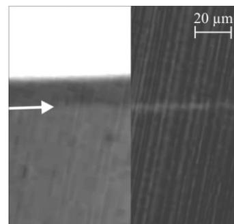
**Figure 10.** Left panel: Optical microscopy reflection image of a device without bias. The white area is the reflective metal cathode, the arrow indicates the insulator edge. Right panel: Optical microscopy image under forward bias. A narrow line of light appears along the insulator edge. The width of the line is estimated to be about 2  $\mu\text{m}$ .
