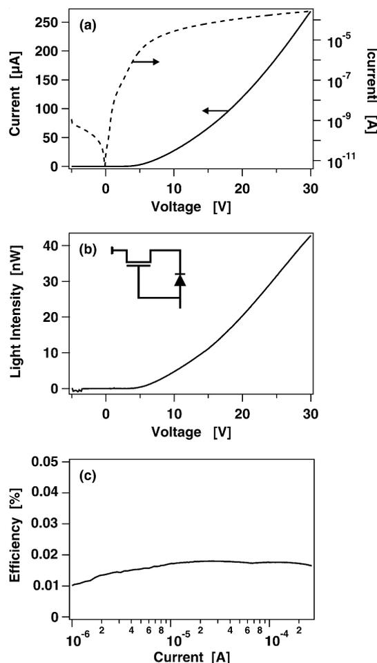
**Figure 8.** Experimentally measured characteristics of the light-emitting diode with field-effect electron transport. This device has a width of 1  $\mu\text{m}$  and a distance between top electrode and insulator edge of 3.5  $\mu\text{m}$ . a) Current–voltage characteristics, b) corresponding light output. The inset shows the equivalent circuit of this device. c) External quantum efficiency of the device as a function of the current.
