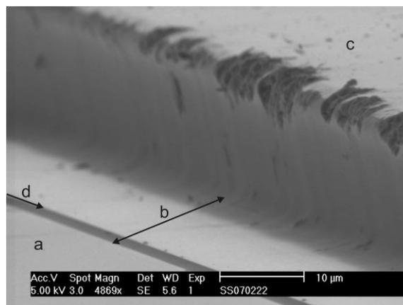
**Figure 3.** Scanning electron microscopy image of the device structure. a) Metallic cathode, b) shadowed region where no metal is deposited, c) the 20 μm thick SU8-25 layer, and d) arrow indicating the insulator edge.
