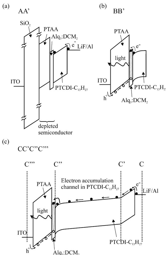
**Figure 5.** Band diagrams for the device under forward bias conditions through different sections of Fig. 1: a) AA', b) BB', and c) CC'C''C''' cross sections.
