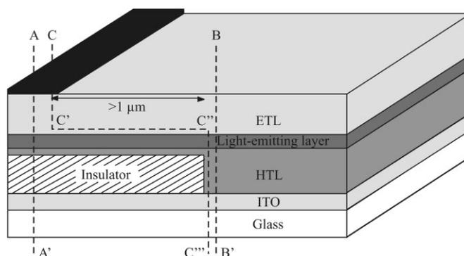
**Figure 1.** Schematic architecture of the OLED exhibiting field-effect electron transport. The device comprises an organic hole-transport layer, an organic electron-transport layer, and an organic light-emitting layer. The dashed lines AA', BB', and CC'C'' indicate three different cross-sections.
