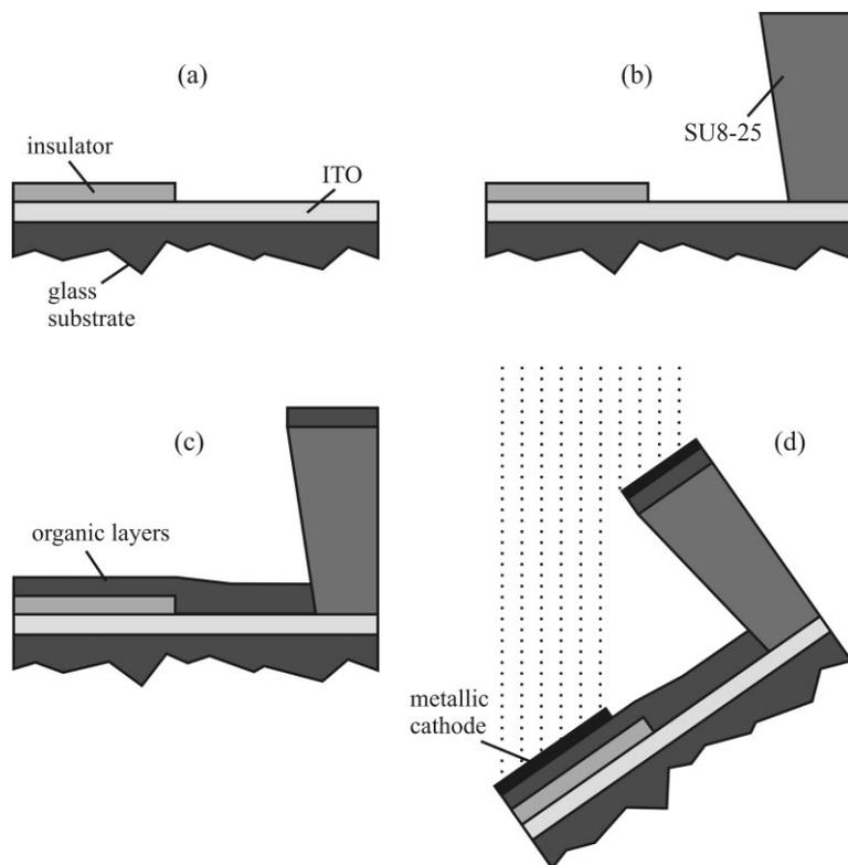
**Figure 2.** Schematic depiction of the processing sequence for the fabrication of the light-emitting field-effect device structure: a) situation before creation of the integrated shadow mask, b) deposition of the integrated shadow mask, c) deposition of the organic layers, and d) deposition of the metallic cathode with the substrate mounted on a triangular sample holder. During this deposition process, the atomic flux is at a 45° angle with respect to the substrate.
