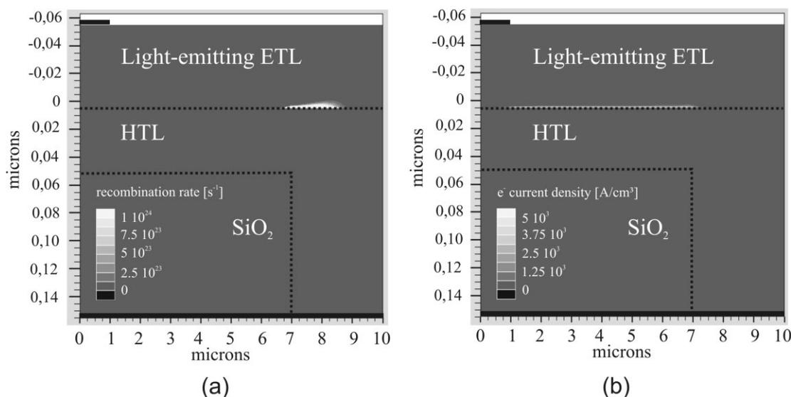
**Figure 11.** a) The simulated recombination rate and b) the simulated electron accumulation layer under forward bias.
