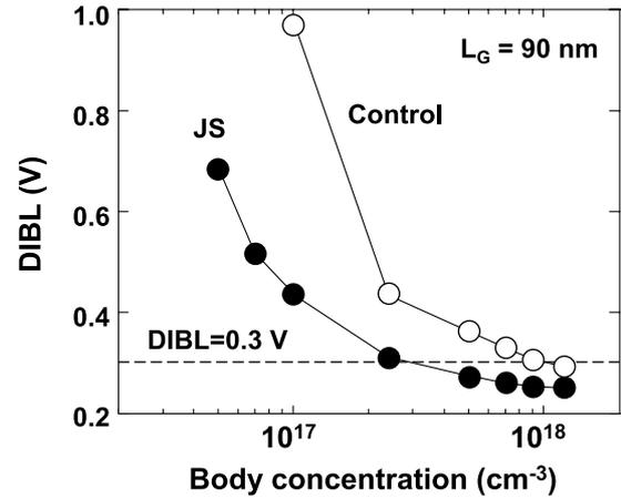
**Figure 5.** Simulated DIBL as a function of the body doping concentration of the JS-VMOSTs ( $L_G = 90$  nm). For comparison, the results of the conventional VMOSTs are also shown. The DIBL values are evaluated from the gate voltage shift in the subthreshold characteristics between  $V_D = -1$  V and  $-0.1$  V, where the gate voltage is defined at  $I_D = -1 \mu\text{A} \mu\text{m}^{-1}$ .
