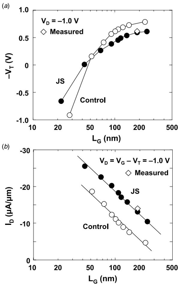
**Figure 4.** (a) The simulated threshold voltage roll-off behaviour at  $V_D = -1$  V of the JS-VMOSTs and the conventional VMOSTs. The measurement result is also included; (b) simulated drain current as a function of channel length of the JS-VMOSTs and the conventional VMOSTs at  $V_D = V_G - V_T = -1$  V. The measurement result is also included.
