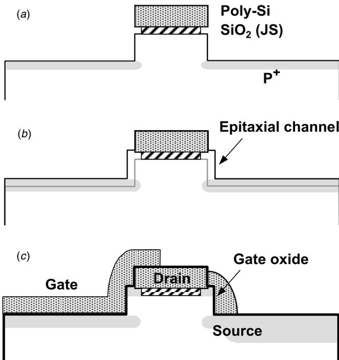
**Figure 1.** Main process steps of a JS-VMOST with an epitaxial channel: (a) formation of a stack of poly-Si and oxide layers, followed by dry etch to form a pillar, boron implantation to form a shallow source junction and HF wet etch to form undercuts on the pillar sidewalls; (b) Si epitaxy for the undoped channel; (c) gate oxidation, gate spacer formation and boron implantation to form a deep source junction. A poly-Si liner extends to one side of the gate spacers for the gate contact.
