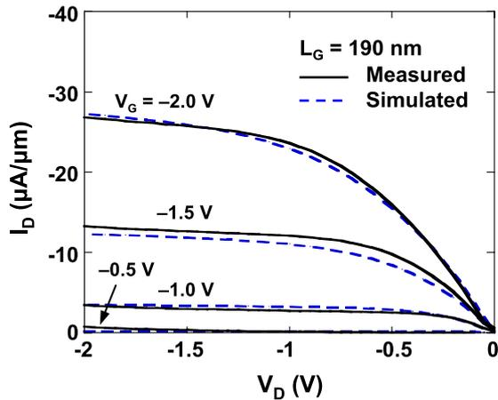
**Figure 3.** Measured and simulated output characteristics of the JS-VMOST ( $L_G = 190$  nm).
