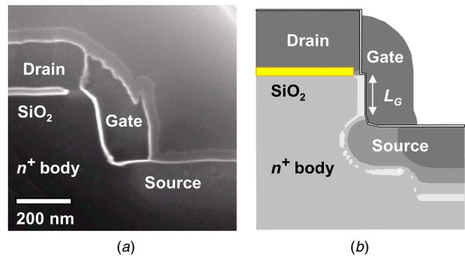
**Figure 2.** (a) Cross-sectional SEM image of the JS-VMOST after junction stain etch; (b) a corresponding simulated device structure.
