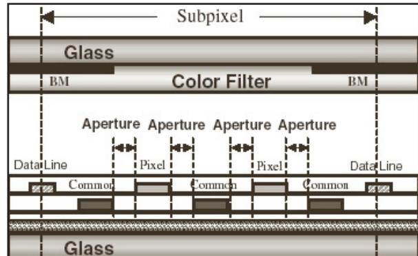
Figure 1. Conventional IPS mode TFT-LCD vertical structure(5).
