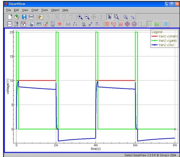
Figure 6. SmartSpice simulation of a pixel.
