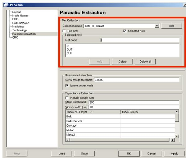
Figure4. Setup of the selective net extraction in Guardian LPE.
