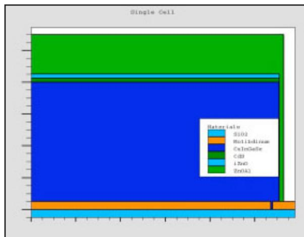
Figure 2: CIGS single solar cell structure.
