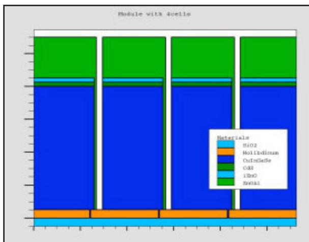
Figure 1: CIGS Solar cell module including 4 cell.
