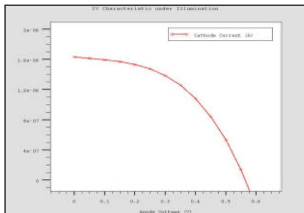
Figure 3: CIGS single solar cell IV curve.
