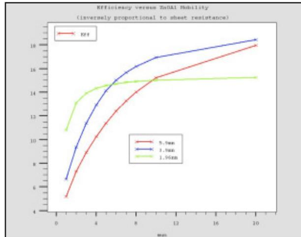
Figure 7: Module Efficiency versus ZnO:Al Mobility.
