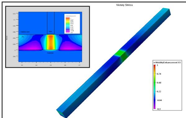
Figure 3. The Mobility Enhancement in the XX direction, along the axis of the silicon fin. Inset: The XX Mobility Enhancement in a cut plane through the active region.
