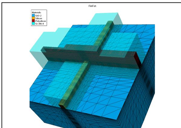
Figure 1. The FinFET structure generated by VICTORY CELL. The  $\text{Si}_3\text{N}_4$  layer is shown transparent in order to display the Silicon Fin and Polysilicon Gate underneath.
