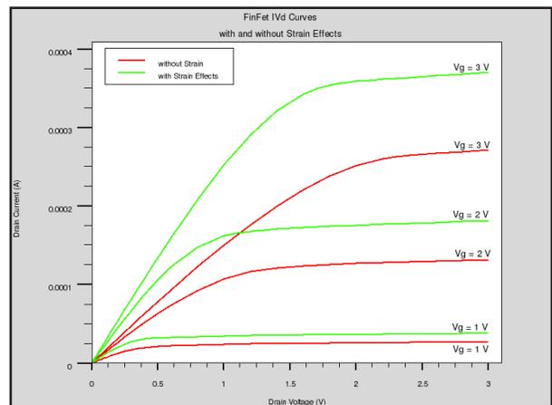
Figure 5. The IV curves for the FinFET simulated with and without strain effects.
