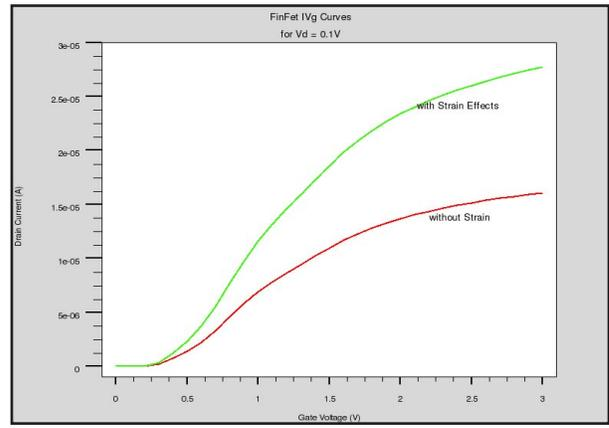
Figure 4. The drain current of the FinFET at  $V_{\text{drain}}=0.1\text{V}$  for gate Voltages ranging from 0 to 3V.
