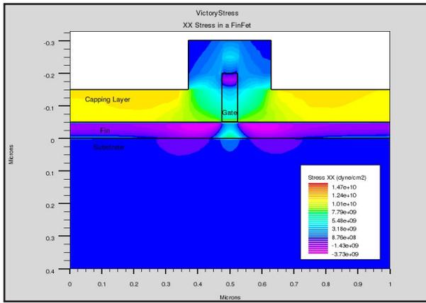
Figure 2. The XX strain in a cut-plane along the center of the device.
