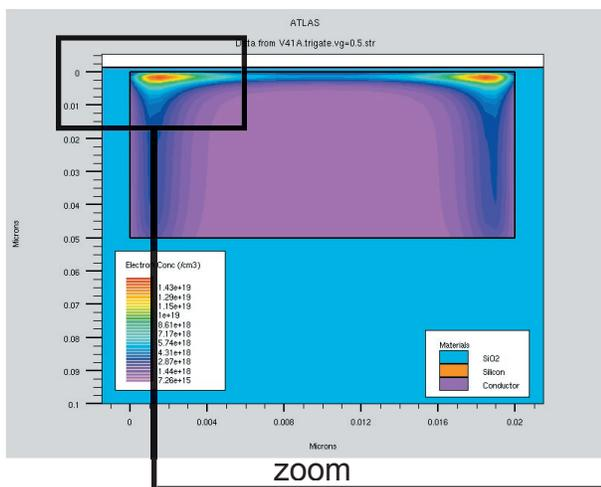
Figure 2 show electrons concentration in linear scale at Vgate=0.5V
