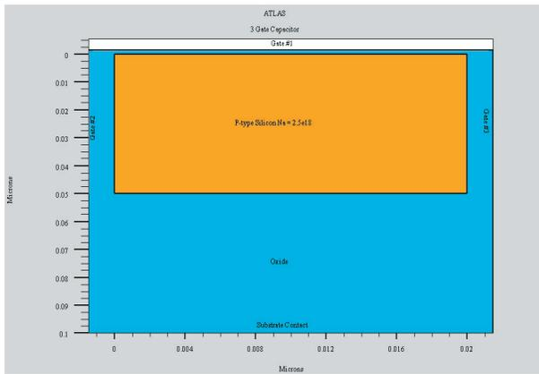
Figure 1. 3 gate capacitor.
