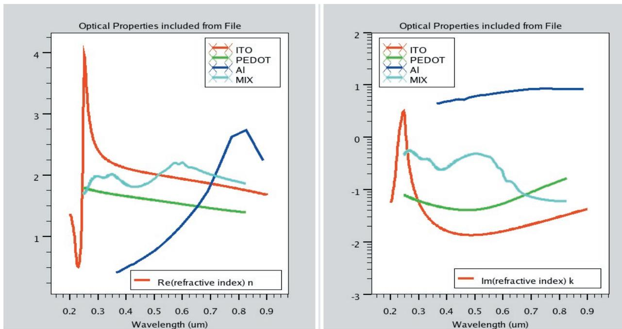
Figure 2. Optical Properties of layer materials used in the simulation.
