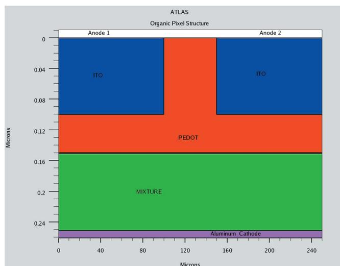
Figure 1. Device Structure – Neighboring Pixel. Note the very different scales along the horizontal and vertical directions.
