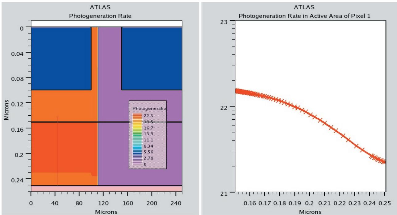
Figure 3. Illuminated Device: Photogeneration Rate along cutline in the illuminated Pixel.
