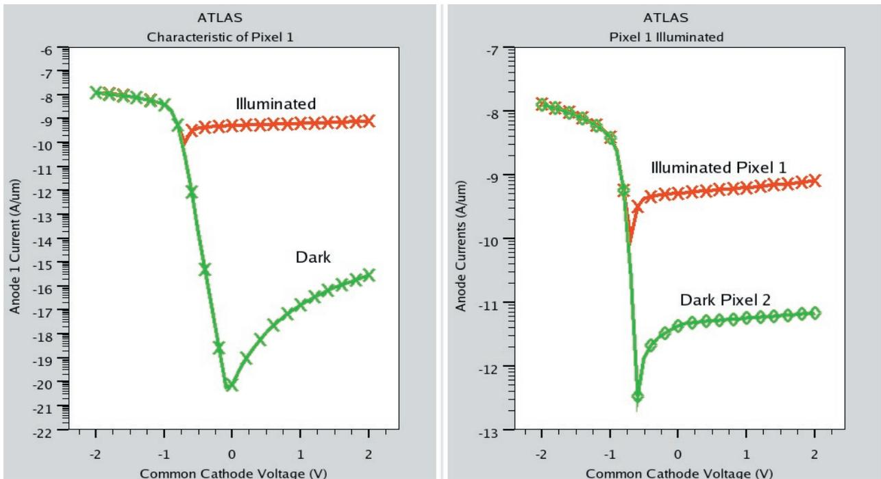
Figure 4. IV Characteristics of Pixels. Only Pixel 1 is illuminated homogeneously with light of 550 nm wavelength.
