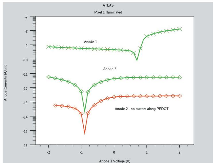
Figure 5. Anode currents for the two neighboring pixels. Pixel 1 is illuminated. The common cathode is grounded. The red curve is calculated for a device with a thin dielectric layer to separate the two pixels electrically along the PEDOT layer.
