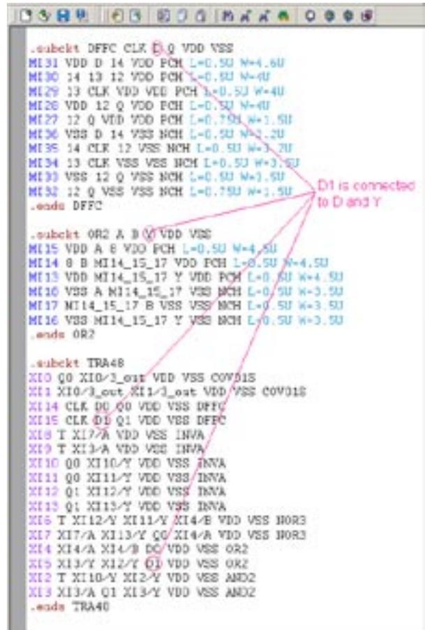
Figure 1a. The part of hierarchical netlist. Netlist corresponds to layout on Figure 1 b,c,d.
