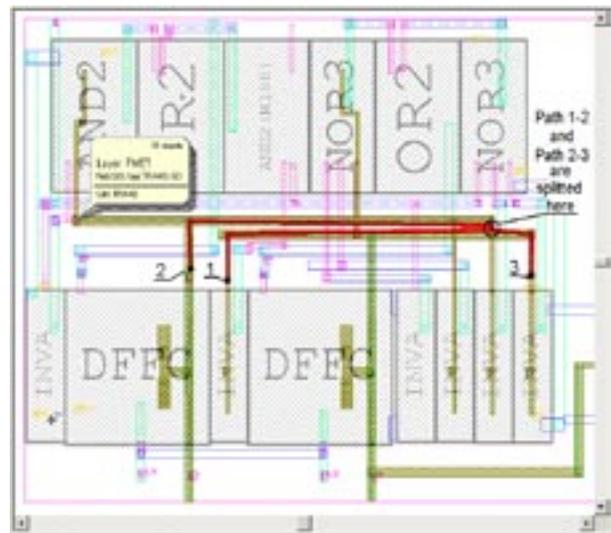
Figure 3d. Shortest paths between points 1,2 and 2,3. Shortest paths are splitted in the place of the short.
