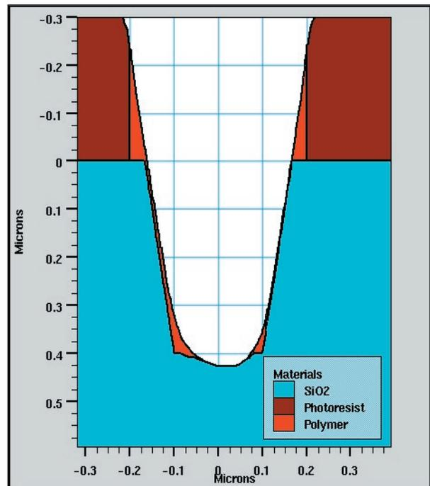
Figure 2. The result of oxide trench etch.
