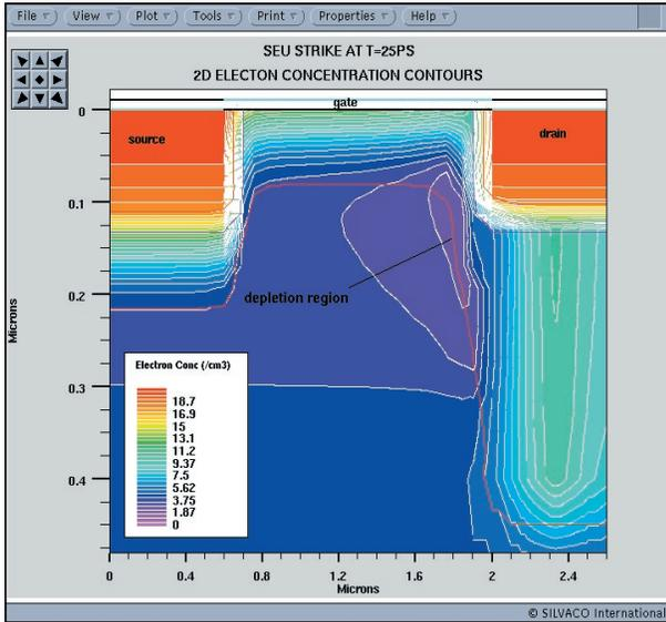
Figure 3. 2D Contours of electron concentration during the particle strike.
