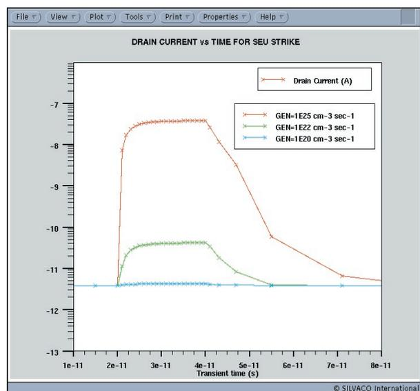
Figure 2. Simulated drain current versus time for 3 separate particle strikes. The generation rate (or particle energy) was varied as
