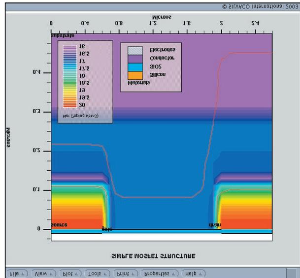
Figure 1. Simple 2D MOSFET structure for the alpha particle strike simulation. The drain bias is 3.3V so the depletion regions extend into the bulk as shown.
