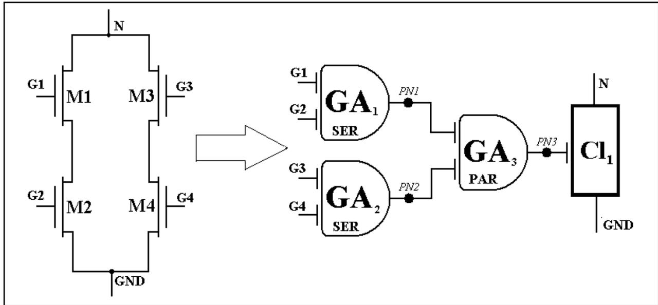
Figure 5. Reduction for parallel-series network realized in Guardian LVS tool.
