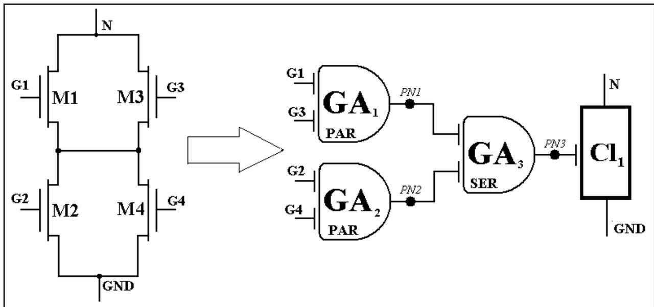
Figure 6. Reduction for series-parallel network realized in Guardian LVS tool.
