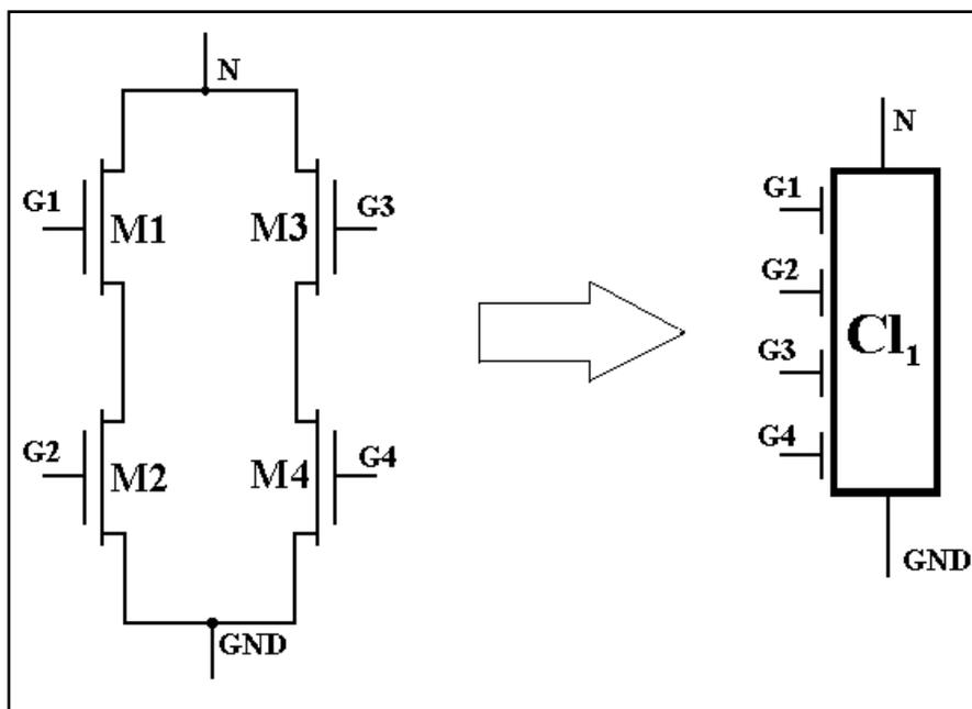
Figure 4. Reduction for parallel-series network using simple abstraction model.
