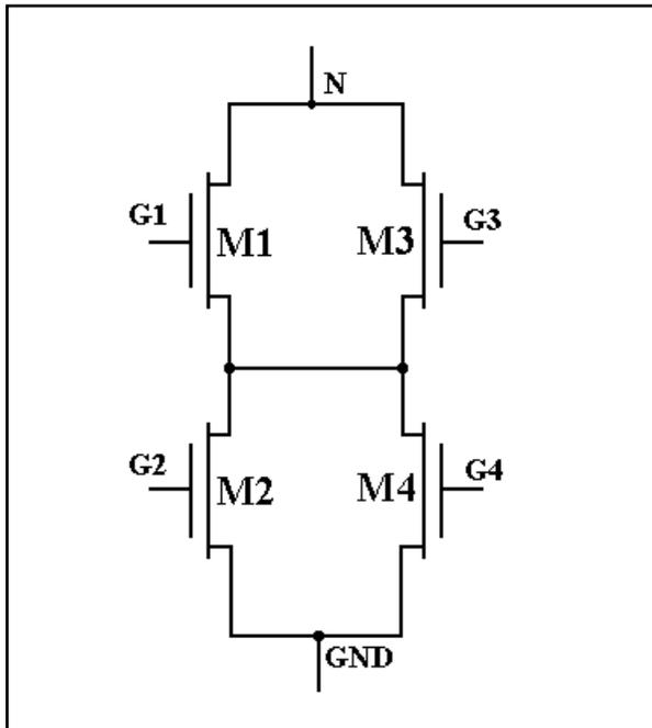
Figure 2. Series-parallel network of MOSFET transistors.
