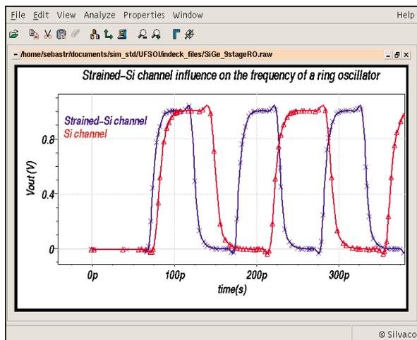
Figure 6. strained- and unstrained-Si devices ring oscillator.
