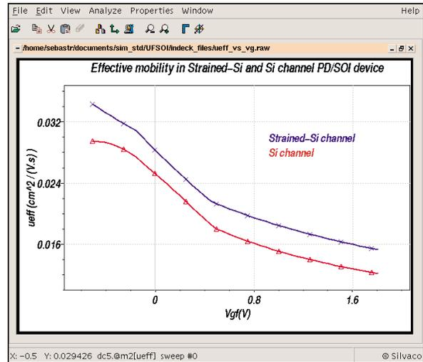
Figure 5. Field-effect mobility with strained- and unstrained-Si channel on a L = 60nm device.
