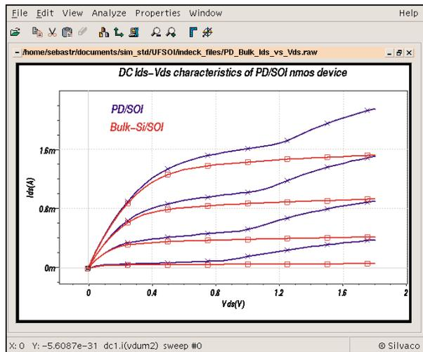
Figure 1. Ids vs Vds characteristics in PD and Bulk-Si mode of the UFPDB model.
