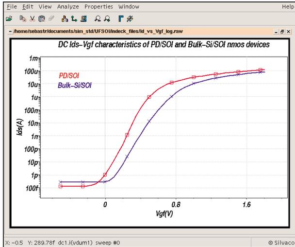
Figure 2. Subthreshold characteristics in PD/NFD and Bulk-Si mode.
