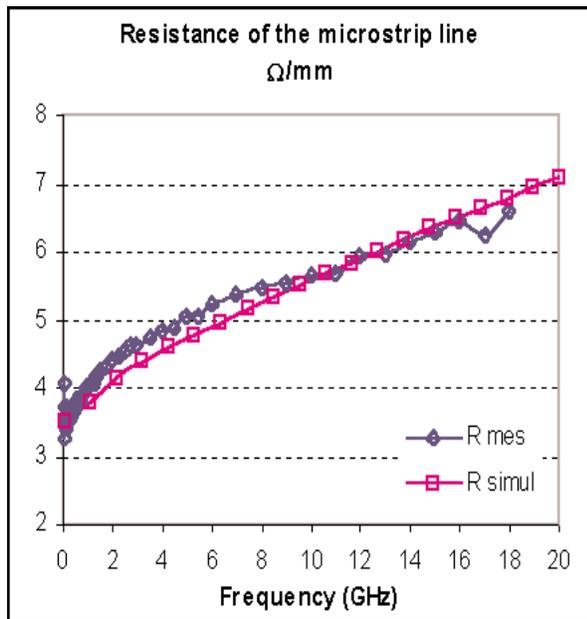
Figure 4. Comparison of measured and simulated resistance.
