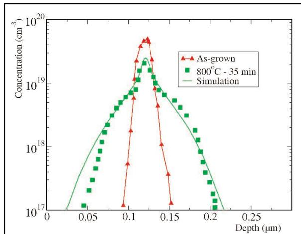
Figure 5. Comparison between experimental and simulated B profiles evidencing the influence of the BIC's. Data are from ref.[9]
