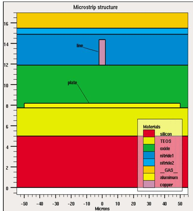
Figure 1. The microstrip structure.
