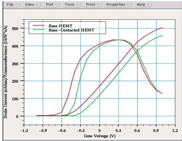
Figure 6. Subthreshold characteristics for base and body-contacted HEMT structures. Characteristics extracted at  $V_D = 2V$ .
