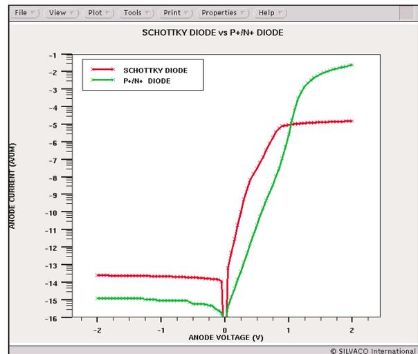
Figure 2. Simulated IV characteristics of the Schottky and pn diodes.
