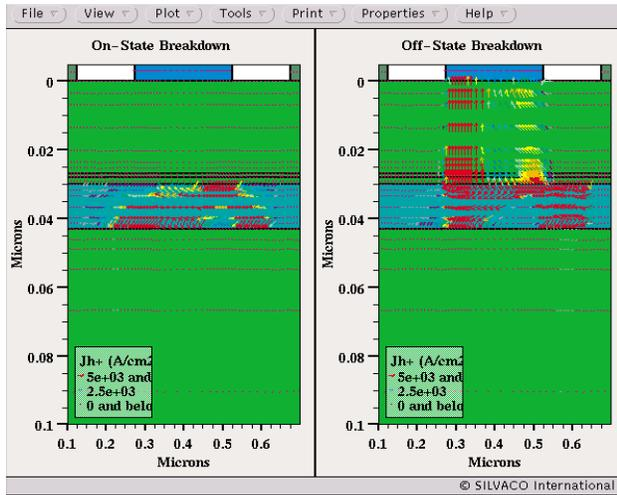
Figure 5. Hole current density vectors for the body-contacted HEMT under a) on-state breakdown ( $V_G = 0.8V$ ,  $V_D = 7V$ ) b) off-state breakdown ( $V_G = -0.4V$ ,  $V_D = 15V$ ).
