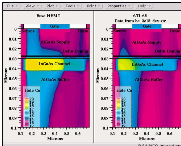
Figure 3. 2D device cross section taken from base and body-contacted HEMT structures with overlain contours of hole concentration ( $\text{cm}^{-3}$ ).
