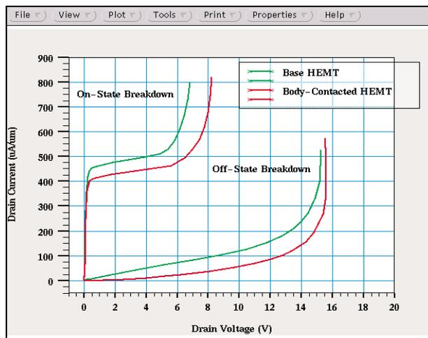
Figure 2. Simulated HEMT breakdown characteristics for both the Base and Body-Contacted HEMT structures. On-state simulations conducted at  $V_G = -0.4$  V; Off-state simulations conducted at  $V_G = 0.8$  V.
