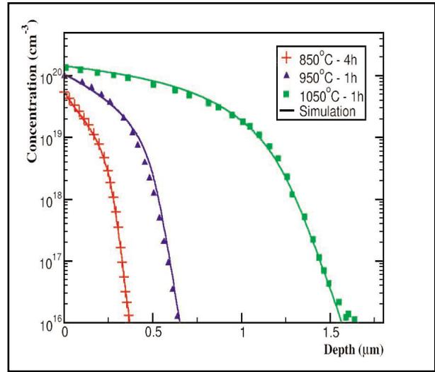
Figure 1. Comparison between calculated and experimental boron predeposition profiles. Experimental data are from ref. [4]
