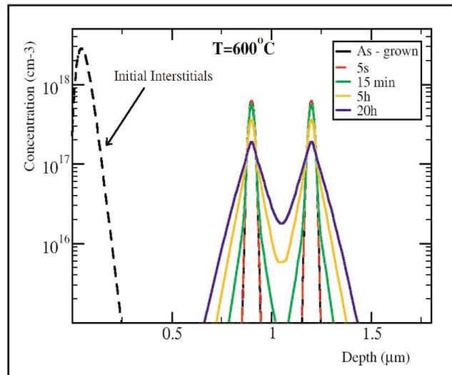
Figure 3. Comparison between experimental and calculated I supersaturation (a), and corresponding calculated B profiles corresponding to ref.[7] (b)
