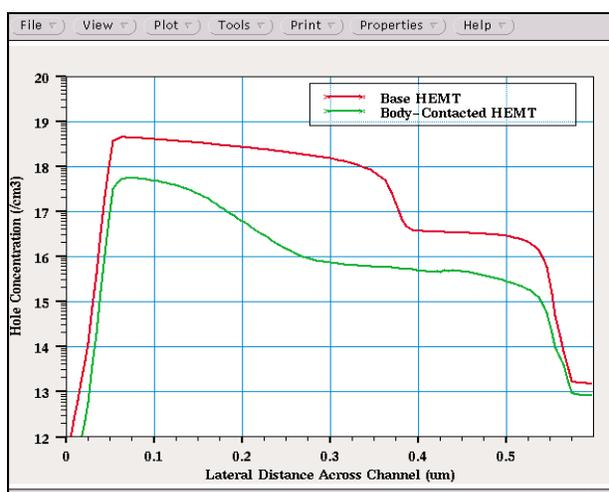
Figure 4. Hole concentration across device channel at on-state breakdown
