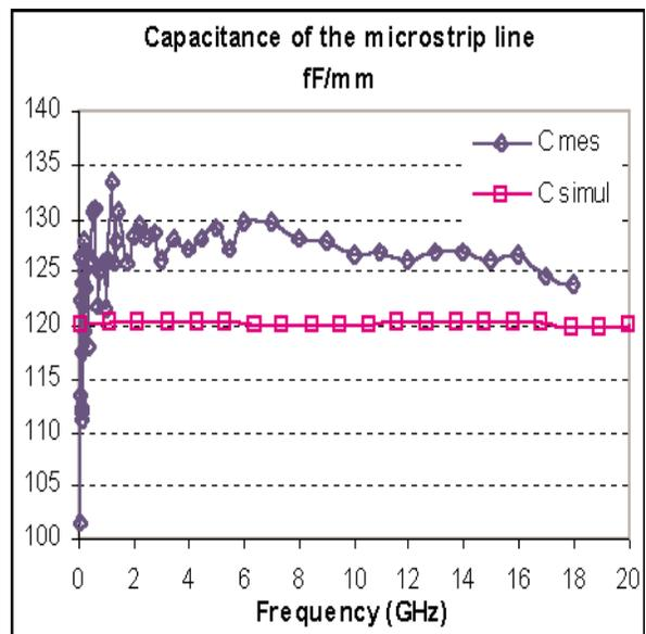
Figure 6. Comparison of measured and simulated capacitance.
