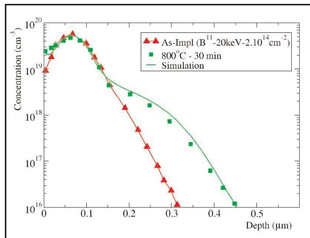
Figure 6. Comparison between experimental and simulated B profiles implanted at  $20 \text{ keV} / 2.1014 \text{ cm}^{-2}$ , annealed at  $800^\circ\text{C}$  for 30 min.
