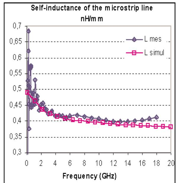
Figure 5. Comparison of measured and simulated self-inductance.
