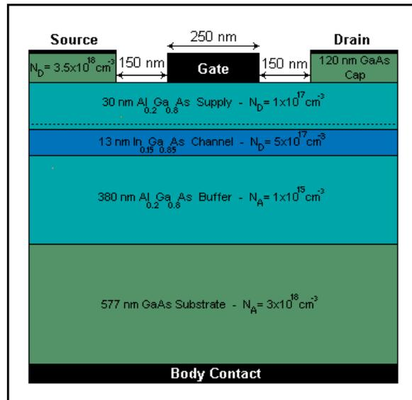
Figure 1. Schematic cross section of the simulated submicron pseudomorphic body-contacted HEMT
