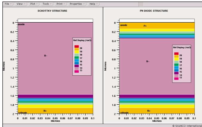
Figure 1. The structures simulated were a Schottky diode and a pn diode. In the Schottky case the anode contact was the Schottky contact.
