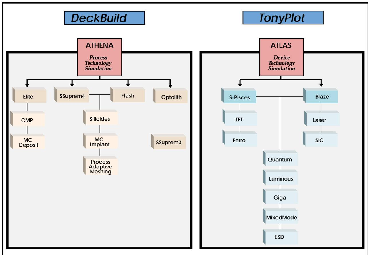
Figure 1. Products available in the Fall 99 release of PC-TCAD.
