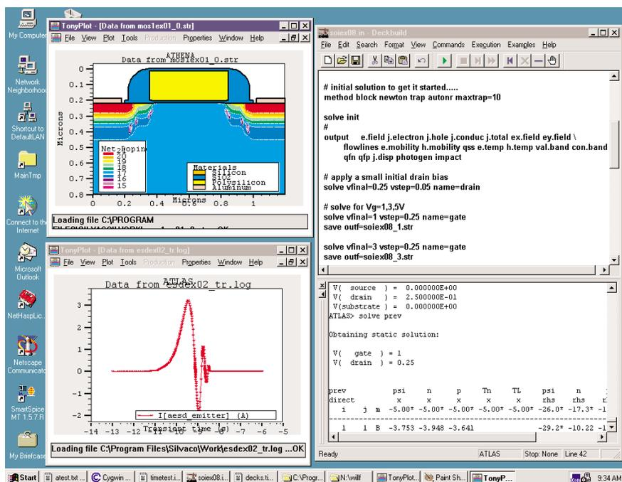
Figure 2. Screenshot of the PC-TCAD Interactive tools DeckBuild and TonyPlot.
