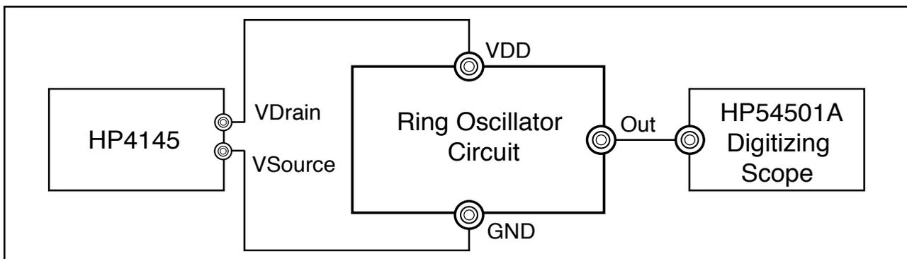
Figure 1. Typical measurement setup for measuring propagation delay of a ring oscillator on a wafer or using a packaged part.
