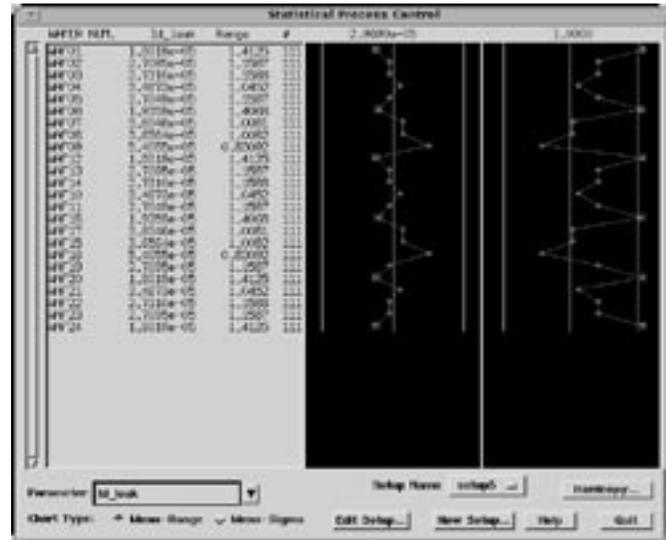
Figure 1. Statistical process control chart for leakage current as a function of wafer number.
