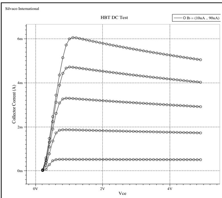
Figure 1. Ic versus Vc plot, illustrating the effect of self-heating.
