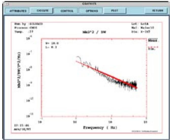
Figure 1. Measured versus simulated Flicker Noise characteristics.
