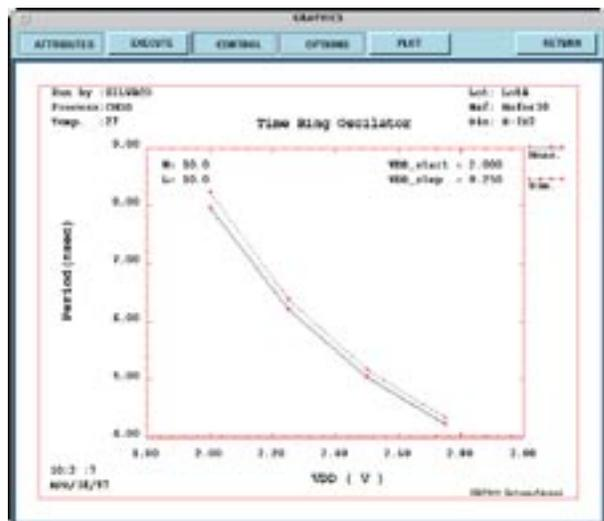
Figure 3. Measured versus simulated data of a 21 stage ring oscillator.
