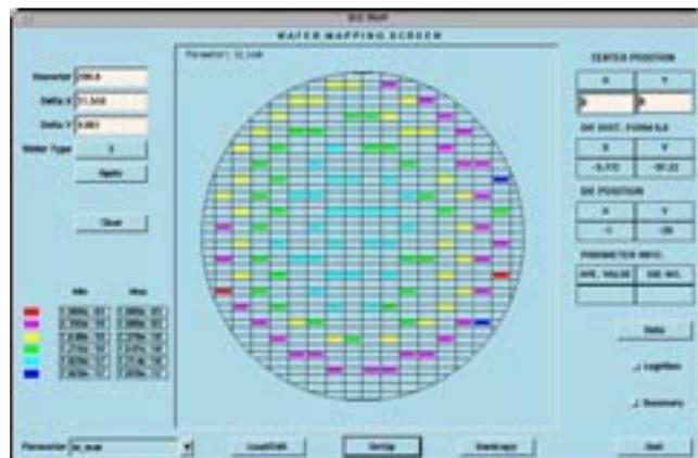
Figure 3. Wafer Map display showing distribution of leakage current.
