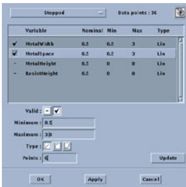
Figure 4: Design of Experiments setup menu for EXACT. DOE setups may be saved and loaded from the EXACT data manager.
