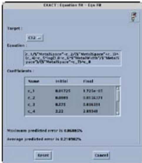
Figure 6 :EXACT fits pre-defined or user generated equations to the raw data.Coefficients in the equations are optimized to provide the best fit
