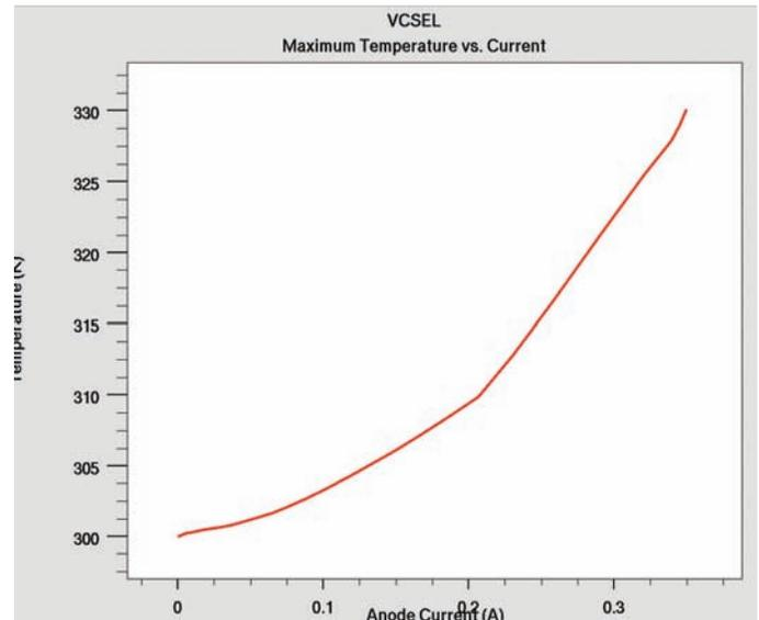
The heat flow equation can also be solved self-consistently to examine the effects of self heating. In this figure we show a plot of the maximum temperature versus the device current.
