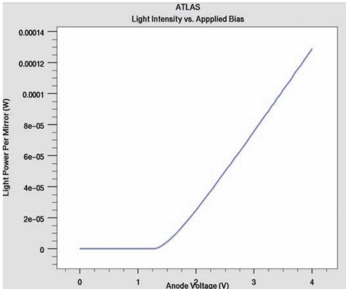
The photon rate equation is solved self-consistently with the device equations to determine the output optical intensity as a function of device bias.
