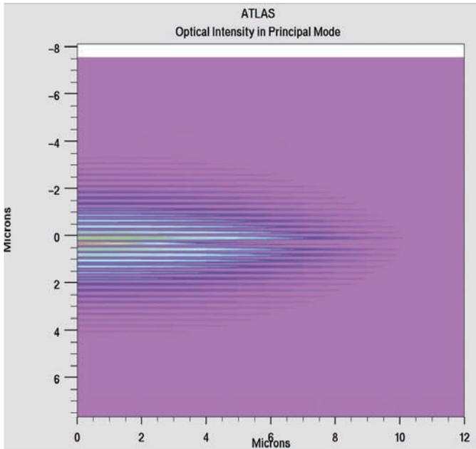
Optical intensity of the principal longitudinal and transverse mode. This mode is lasing at the designed wavelength.
