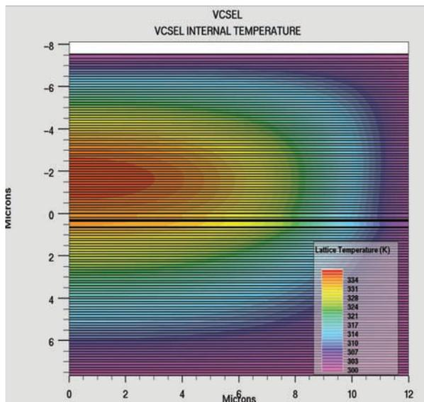
Lattice temperature contours inside the VCSEL at lasing. The temperature dependence of material parameters such as refractive index are included to examine the effects of self heating on optical behavior of the VCSEL.
