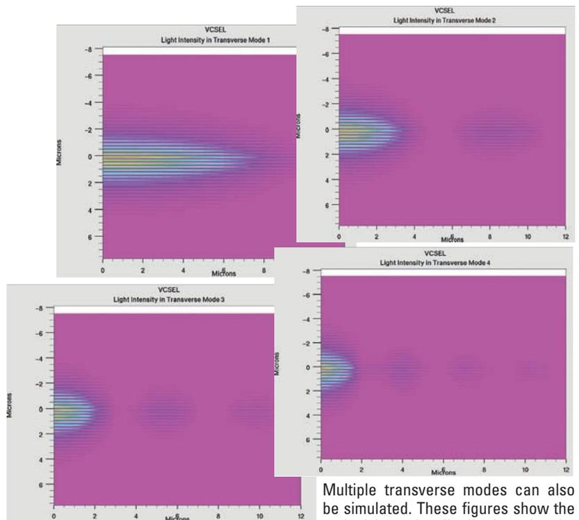
Multiple transverse modes can also be simulated. These figures show the optical intensity distributions for the first four transverse modes of a typical VCSEL.
