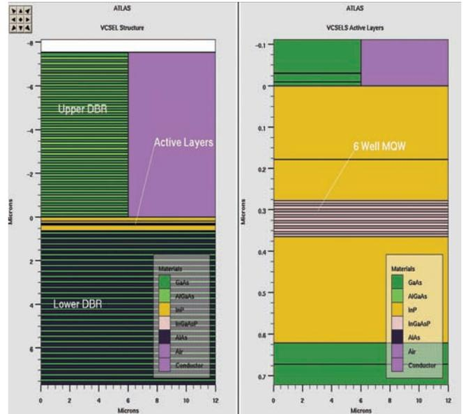
Cross-section of a typical VCSEL device. On the left we see the entire cross-section which shows both the upper and lower DBRs and the active layers. The right panel shows the enlarged cross-section around the active layers where we can see that this device contains a six layer multiple quantum well.
