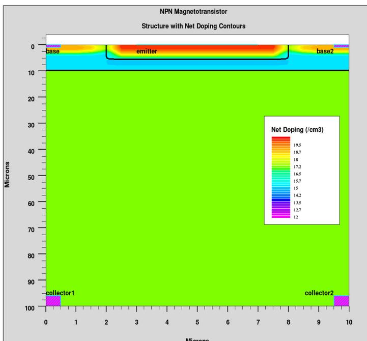
A simple NPN magnetotransistor structure showing net doping contours and the position of the p-n junctions. It is biased in a common emitter arrangement, with 10 V bias applied to the collector contacts. The base contacts are then biased from 0.0 V to 0.65 V. Results are obtained without a magnetic field and also with a uniform magnetic field of 1 Tesla applied perpendicular to the device.
