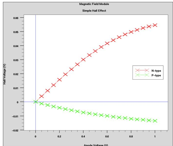
Shows the Hall voltage generated across a simple semiconducting resistor as a function of the bias applied along the resistor. The simulation includes field dependent mobility and the Hall voltage consequently varies sub-linearly with applied voltage. The opposite carrier types give opposite signs for the Hall voltage.
