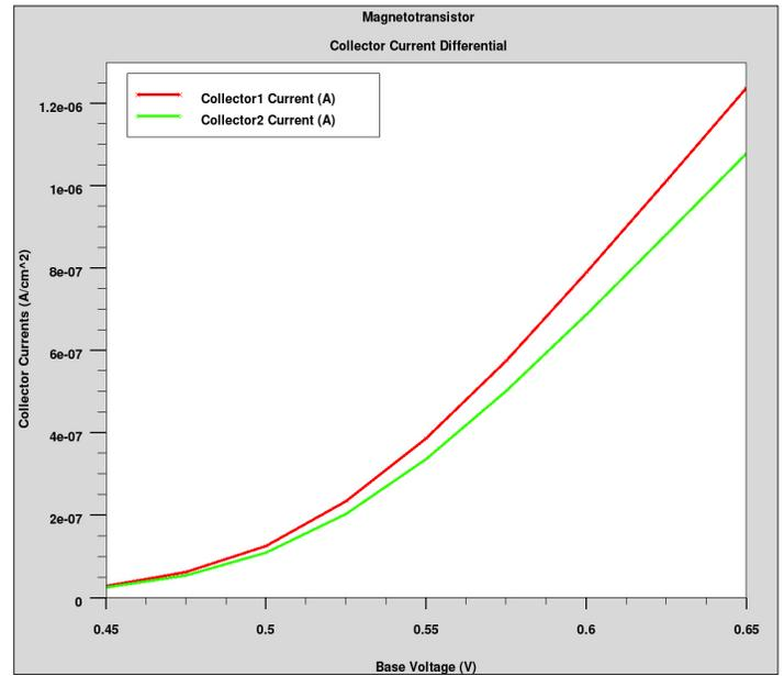
The electron current along the horizontal cutline at 90 microns in the magnetotransistor. Without an applied magnetic field it is symmetric about the device centerline, but the magnetic field gives an asymmetry which results in a current differential between collector 1 and collector 2. This is due solely to the deflection of the current flowlines by the applied magnetic field.
