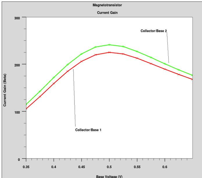
The current gains of the structure, obtained by dividing collector 1 current by base 1 current and collector 2 current by base 2 current. One is enhanced relative to the zero magnetic field case and the other is diminished.
